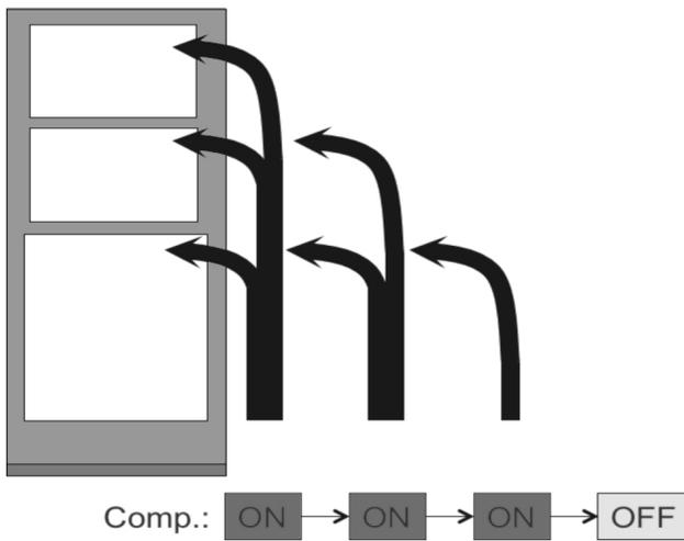
Fig 8.24 Schematic picture over how the distribution of cold air can work with dampers if there are three compartments/zones with different temperatures.
