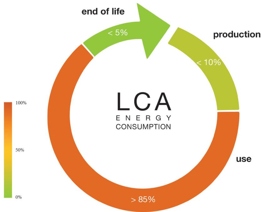
Fig 2.7: Simplified LCA for the energy consumption of a refrigerator during its life time.
