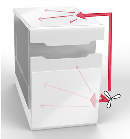
Fig. 9.41: The warm air is directed in the top surface or the side with a DC fan.
