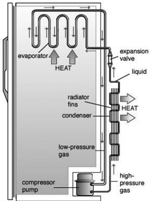
Fig 2.5: Technical principle of a refrigerator with static condenser.
