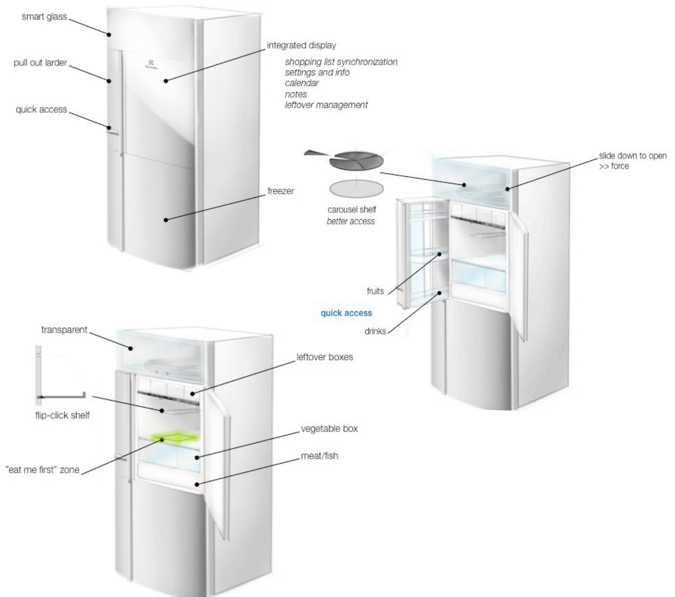
Fig.8.4-6: The Organized, closed and opened with its compartments and features indicated. Inside the top compartment with slide-down-to-open smart glass door, there is carousel shelf. The pull-out larder on the side is for quick access to fruits and drinks. In the large compartment there is an "eat-me-first zone" and a system for post-prepared food.
