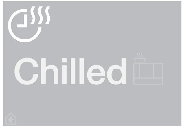
Fig 9.28: The interface for chilling food. When hot food is placed on the top surface the display shows the time it will take before it is chilled enough to be placed in the refrigerator.
