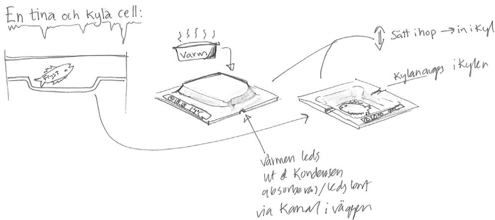
Fig.8.1. Sketches for the concept “the Efficient“, a “double tray” with Peltier cell to insert in the refrigerator to thaw and chill food in
