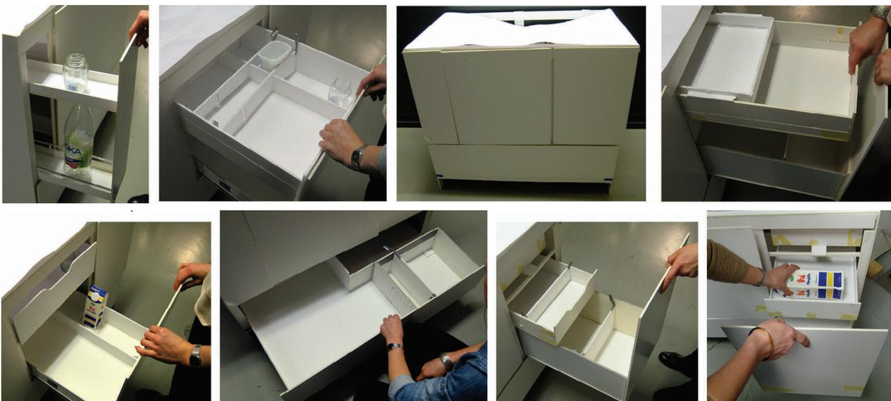
Fig 8.23: The paper mock-up from different views. All the interior parts were built to try dimensions and handling.
