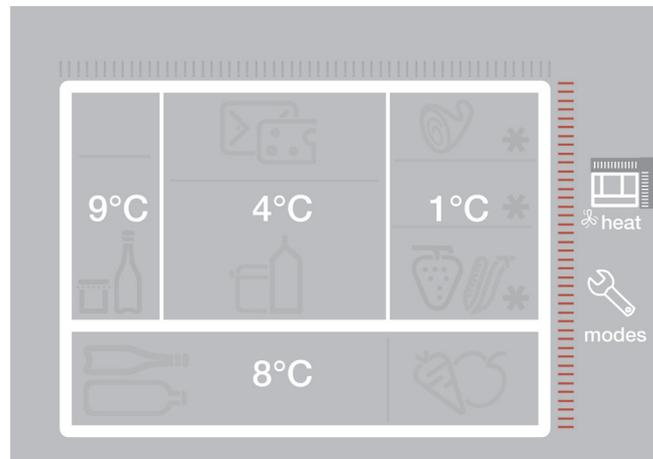
Fig 9.22: This is the first view of the display - all compartments and the present temperature in each. If the temperature deviates from what it should be the numbers are shown in red or blue.
