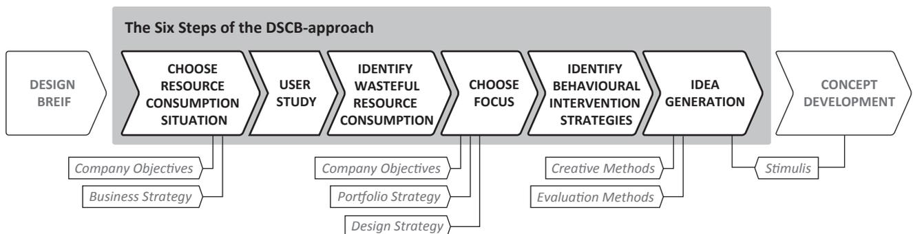
Fig.2.1: The DSCB design process; described in its six steps. (Selvfors, Blindh Pedersen and Rahe, 2011)
