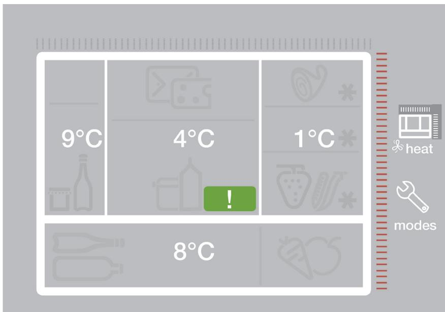
Fig. 9.38: The EatSoonZone is marked in the display if it is well loaded. The “!” denotes there is a notification for someone about something that has to be eaten. The red dashed lines on the sides of the refrigerator icon indicates where the warm air is directed and it can be switched by pressing on it.
