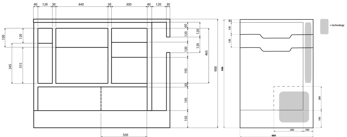
Fig. 9.43: Dimensions of all the compartments of Pompadour.
