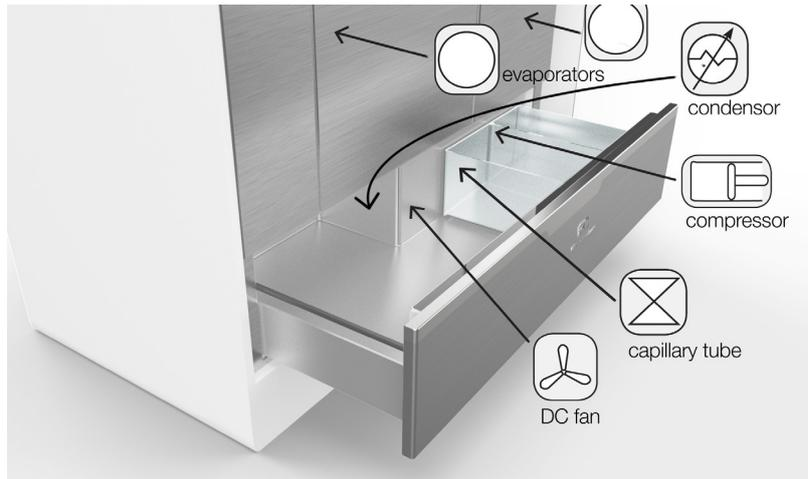
Fig. 9.42: Suggested placement of refrigeration technologies.
