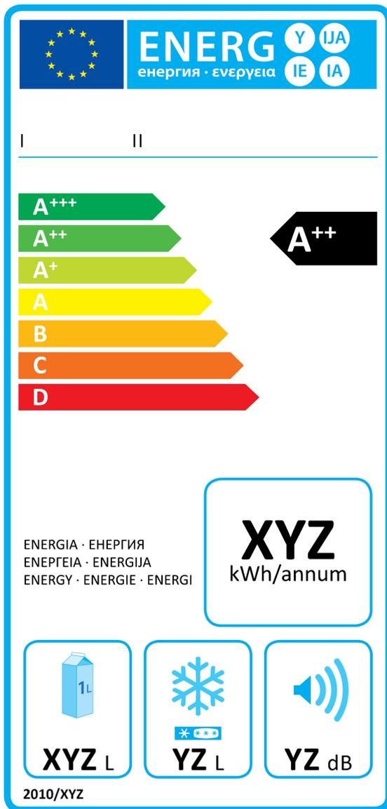
Fig 2.6: The standard energy label. As an example can an A+++ refrigerator of 300 l consume 150 kWh/year, and according to the index an A++ refrigerator consumes 30 % less energy per year compared to an A+ labelled refrigerator and 45 % less than an A labelled appliance.
