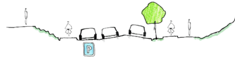
Section of safe and welcoming road suitable for Hjällbovägen. Bikers lane elevated from the pedestrian level. A narrow road, framed with greenery gives a more attractive and varied landscape and keeps drivers alert.
