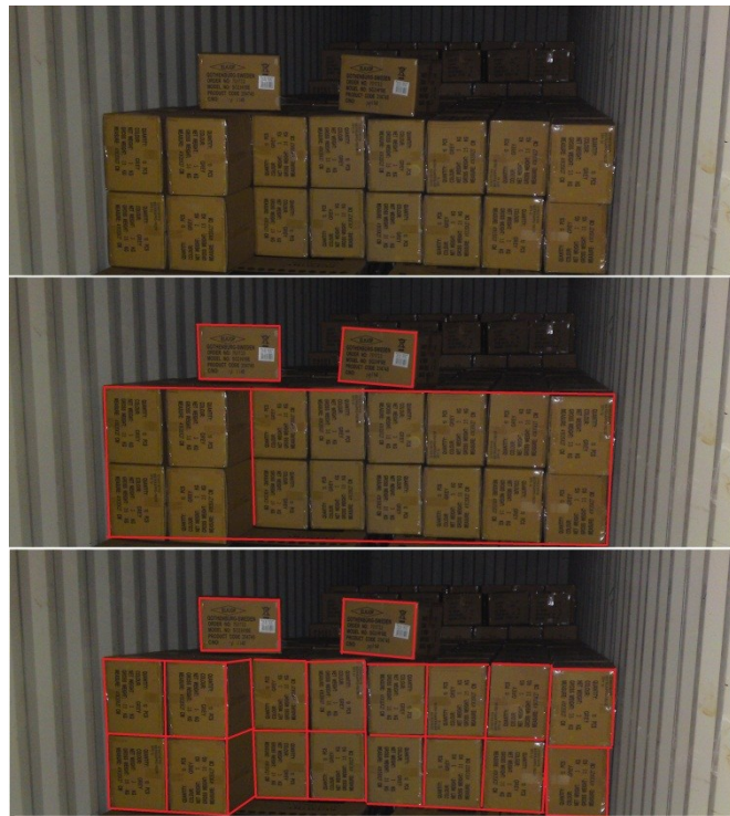
Figure 27: Top, cartons in various orientations in the container. Middle, Geometry of cartons is identified as a whole. Bottom, each box is identified as an entity.
