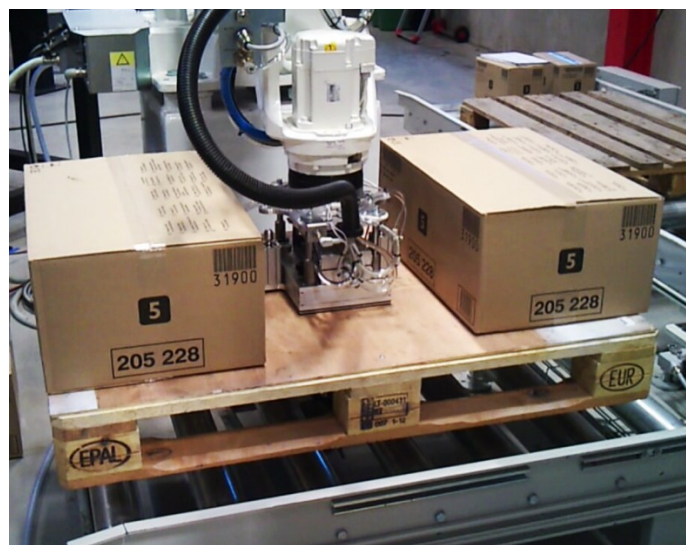
Figure 39: Vacuum gripper successfully lifts pallet weighing fifteen kg and two cartons weighing nine kg each.
