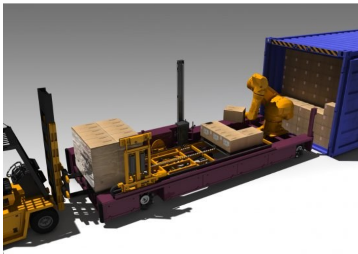
Figure 28: TEUN with integrated unloading, palletizing and wrapping of cartons.
