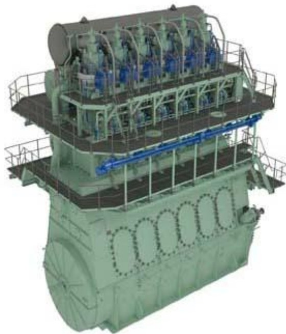
Figure 7-5 Graphical rendering of a MAN B&W 6S70ME-GI engine with gas components shown in blue. Image credit: MAN Diesel & Turbo SE
