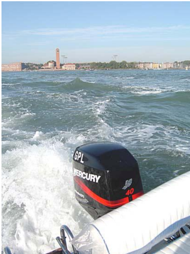
Figure 7-1 The first boat of the demonstration fleet fitted with an LPG/petrol dual fuel engine.
