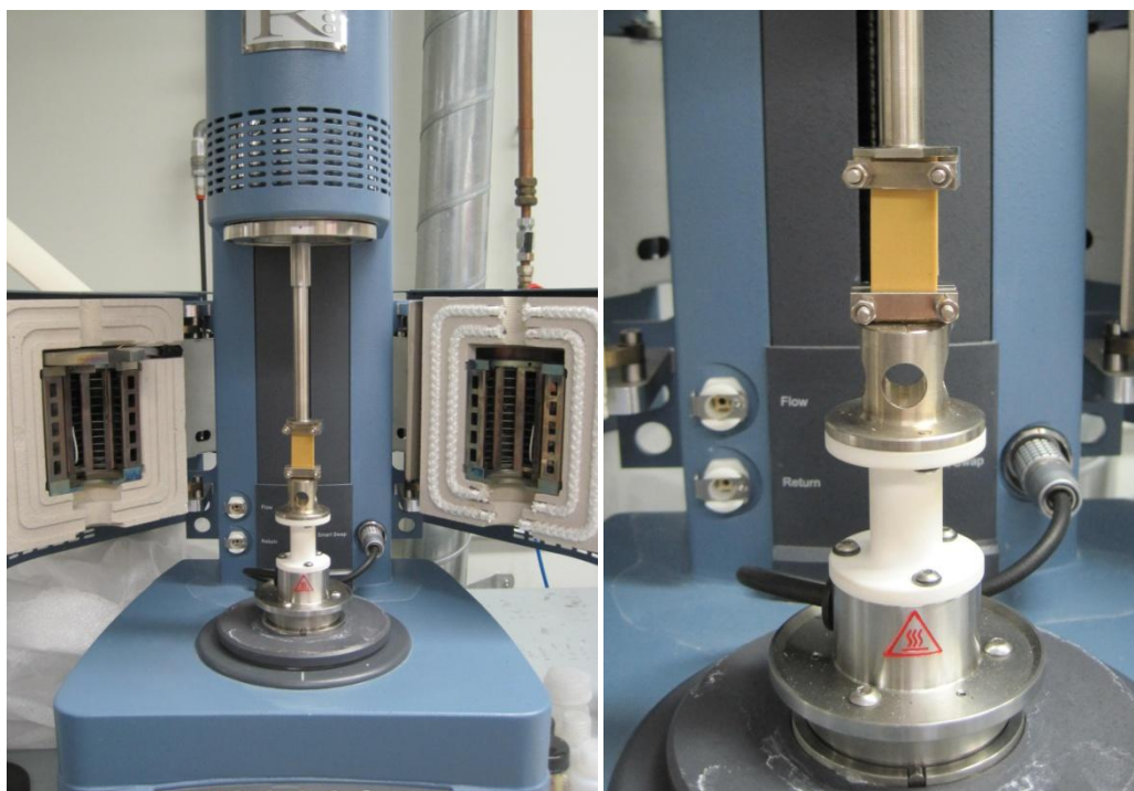
Figure 17. DMTA equipment showing sample B3 attached to the clamps.
