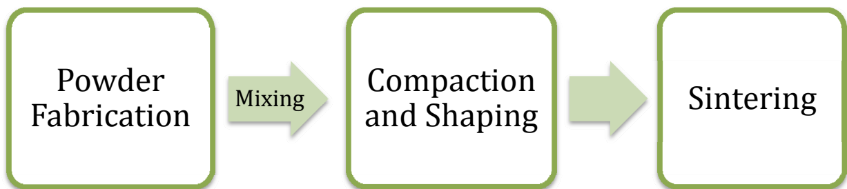
Fig. 4. Chart of the press & sinter PM process route (Author's illustration).
