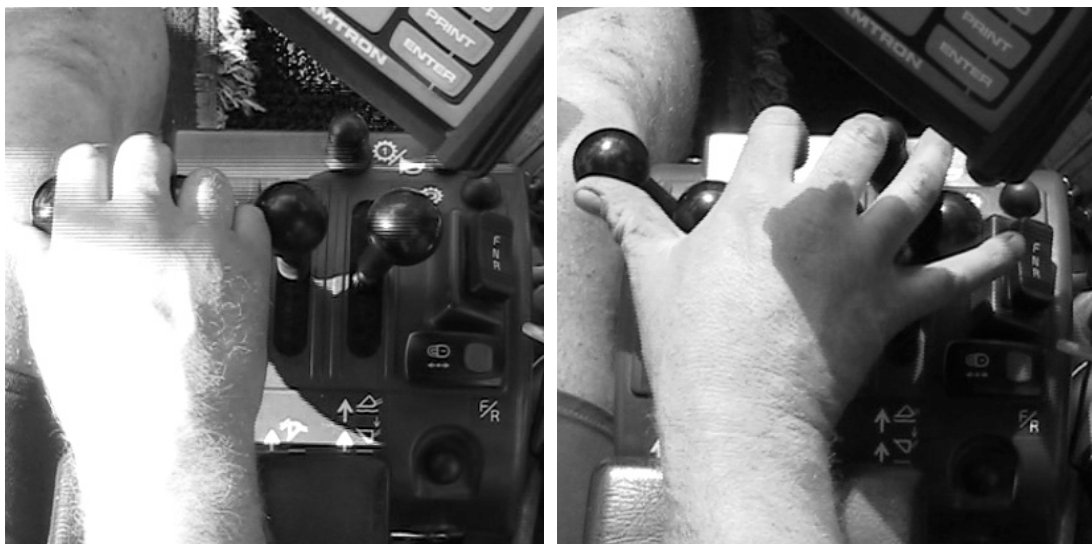
Figure 6.9 working postures of L120F when using all four functions (Snowplow work)
