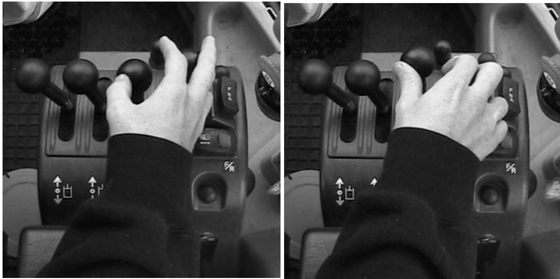
Figure 6.4 working postures of L70F when using 1 st and 2 nd function (Changing attachments)
