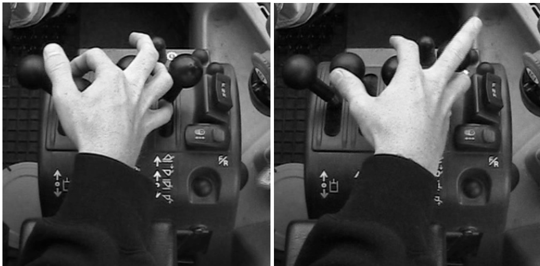
Figure 6.5 working postures of L70F when using 1 st and 2 nd and 3 rd function (Pallet fork work)
