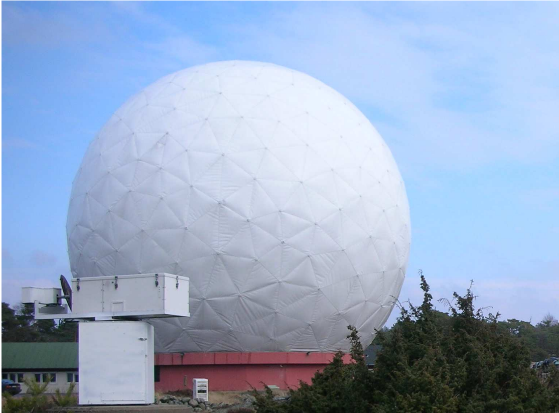
Figure 2.7: The geodetic VLBI site using the 20 m telescope enclosed by the radome at the Onsala Space Observatory. The WVR is seen in the foreground.
