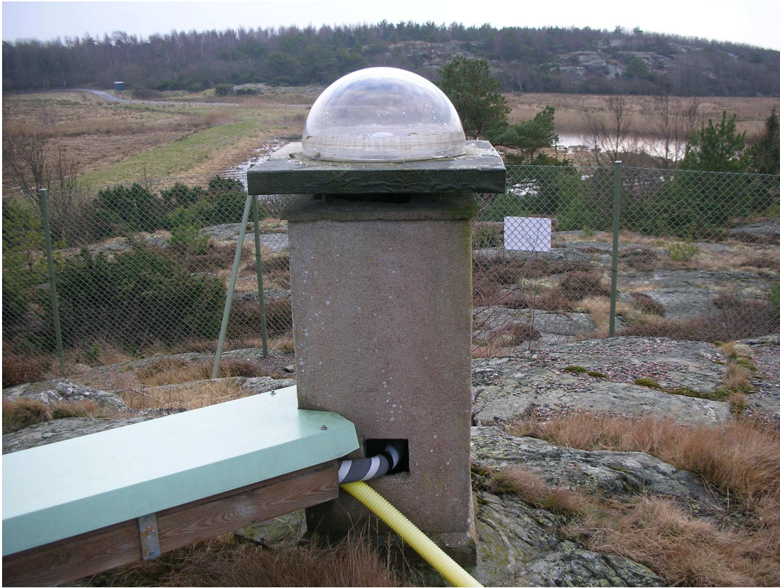
Figure 2.9: The GPS site (ONSA) located at the Onsala Space Observatory is a site in the International Global Navigation Satellite System (GNSS) Service (IGS), formerly the international GPS service, network ( http://igs.cb.jpl.nasa.gov/network/site/onsa.html ). The antenna is protected by a hemispheric radome and microwave absorbing material is attached to the antenna.
