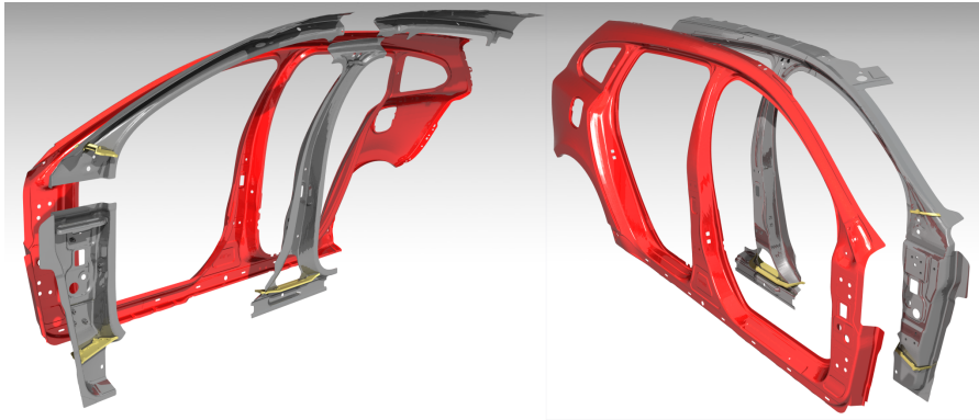
Figure 1.3: Rendered image showing two different views of the car side (red), and the four work pieces (grey) which are welded together and placed onto the car side.
