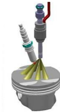
Figure 3.3 – Spray-guided direct injection system used in the multi- & single-cylinder engines.
