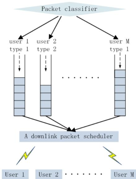
**Figure 1.9:** Structure of the downlink packet scheduling system.
