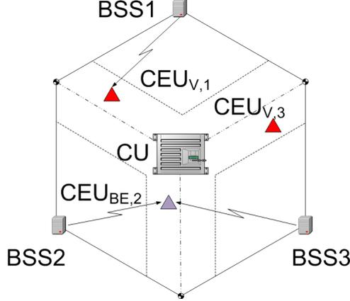
**Figure 2.1:** System model for downlink joint transmission in one CoMP cluster.
