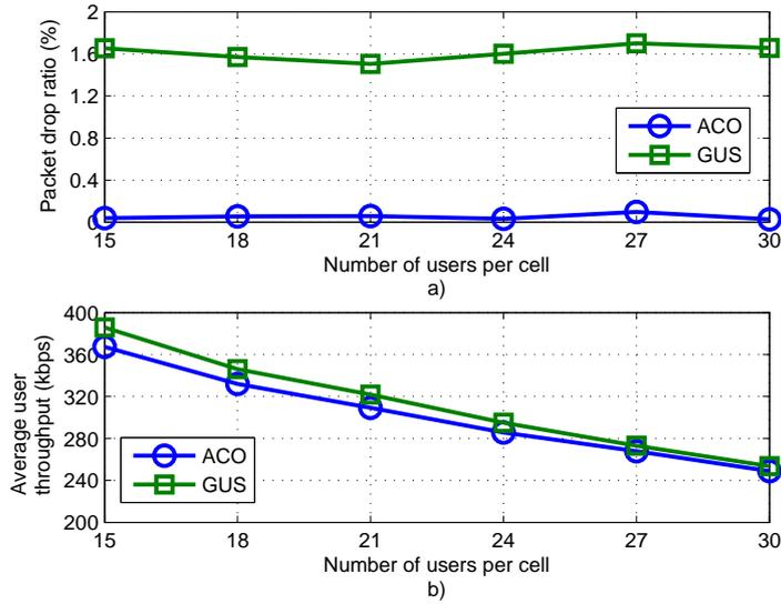
**Figure 3.3:** a) Cell-edge packet drop ratio of VoIP users b) Cell-edge average user throughput of BE users
