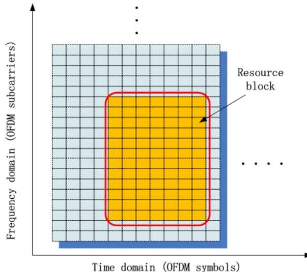
**Figure 1.3:** OFDM time-frequency grid.
