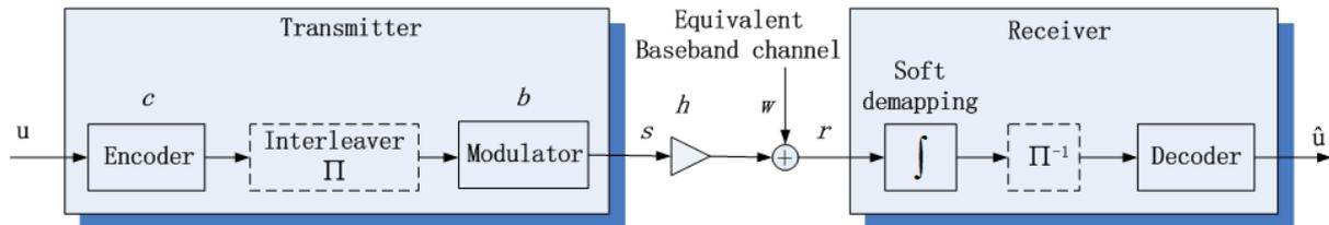
Figure 1.1: Discrete-time system diagram of MCS.
