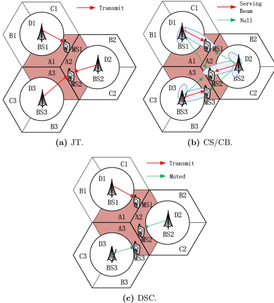
**Figure 1.5:** CoMP downlink transmission schemes. a) JT. b) DCS. c) CS/CB.
