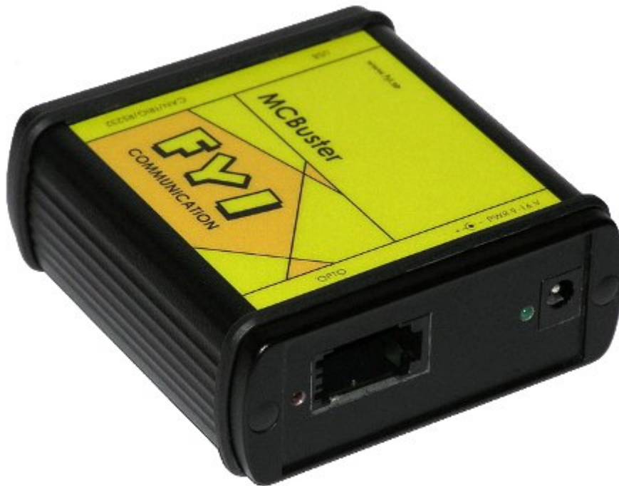
Figure 1: The MCBuster hardware used for MOST analysis. FYI communication www.fyi.se
