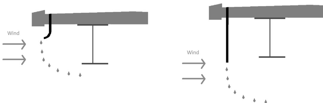
Figure 6.7 Example of two different solutions for the foundational drainage system to avoid that contaminated water blows onto the steel girders
