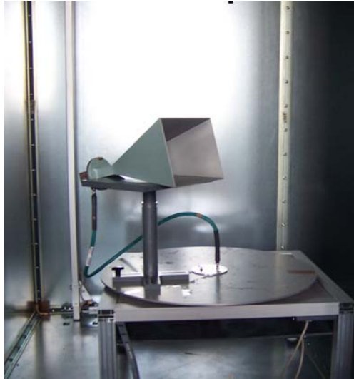
Figure 3.1: Photo of a standard gain horn antenna mounted on the platform in the RC.
