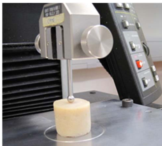
Figure 8. Measurement of gel strength and deformation.
