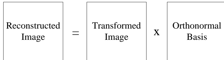
Figure 2.17: the block diagram for reconstruction of an image from its basis images
