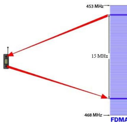
**Figure (4-4):** FDMA in NMT system with 25 kHz separation bandwidth.
