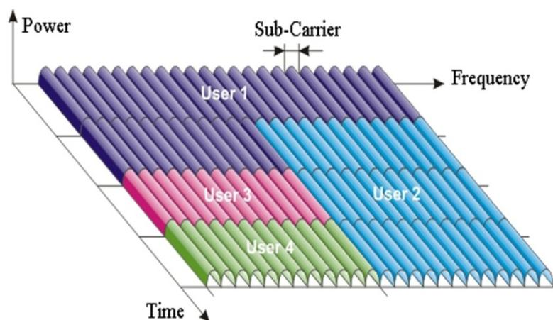
**Figure (3-4):** OFDMA technique in digital transmitting.
