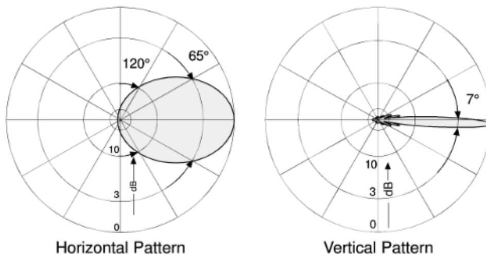
**Figure (2-3):** Radiations from horizontal and vertical directions from the antenna.
