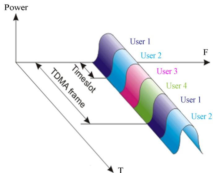
**Figure (3-2):** TDMA technique in GSM cellular systems.
