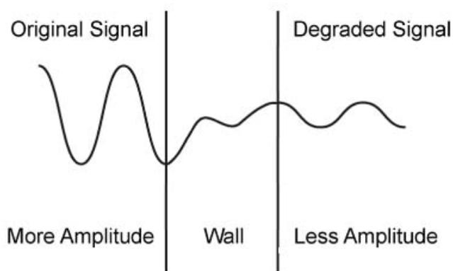
**Figure (2-3):** The example of how path loss affects on the signal by an absorption object.
