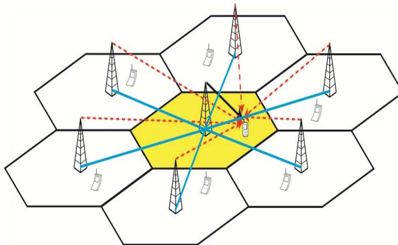
**Figure (4-1):** A cellular system of seven base stations, corresponding to seven different cells.
