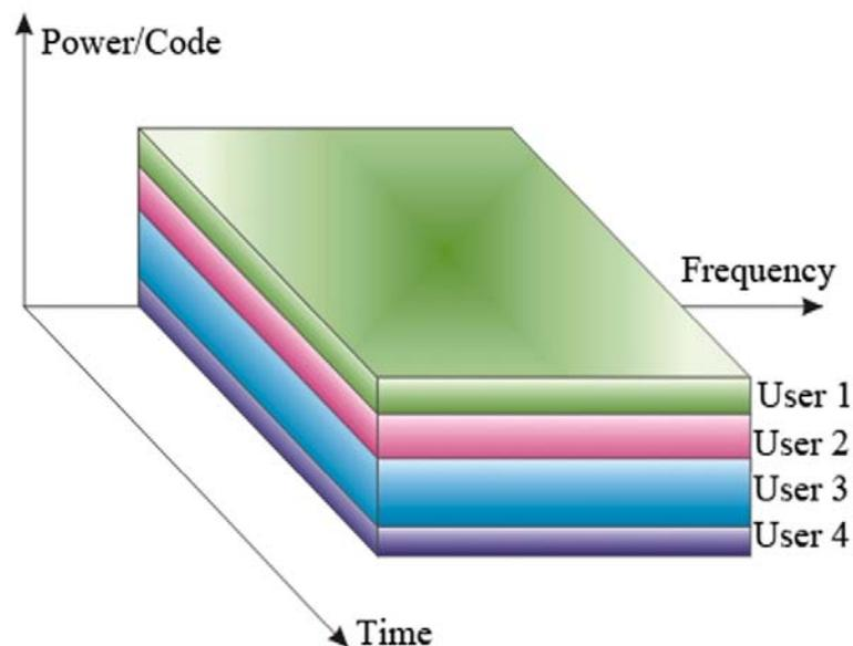
**Figure (3-3):** CDMA technique in wireless commutation.
