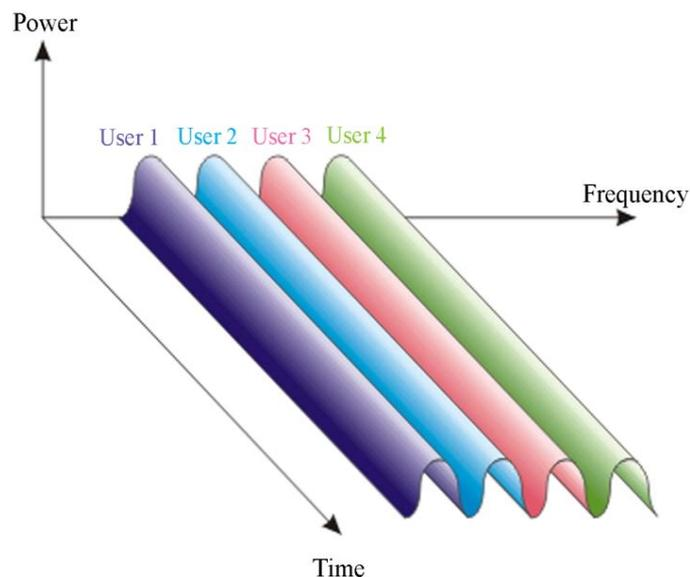
**Figure (3-1):** FDMA with FDD is usually used in analogue cellular system.
