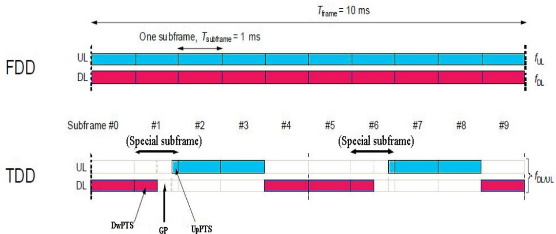
**Figure (4-5):** The LTE frame structure.
