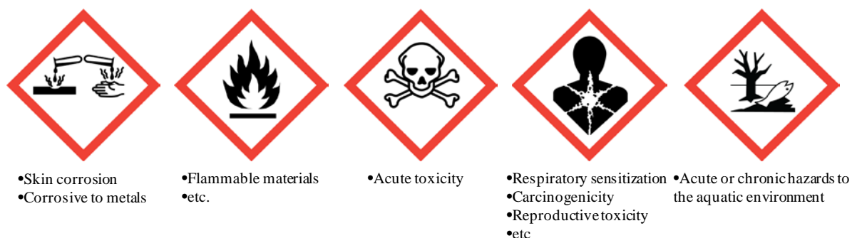
Figure 5 Examples of hazard pictograms according to GHS (United Nations, 2009, United Nations Economic Commission for Europe, 2012)
