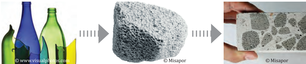
Fig 3: From recycled glass to foam glass aggregates to cellular concrete (with white cement). (based on Misapor, 2011)
