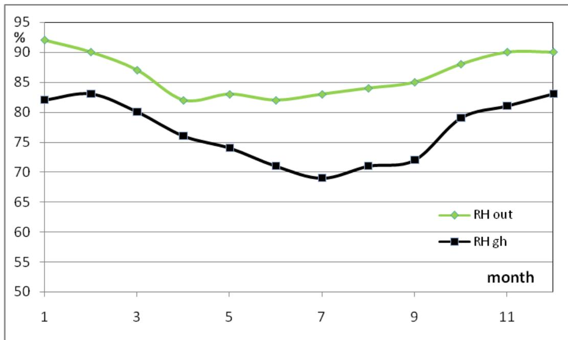
Figure 6.3 Simulated relative humidity in the greenhouse compared to the outdoor relative humidity.
