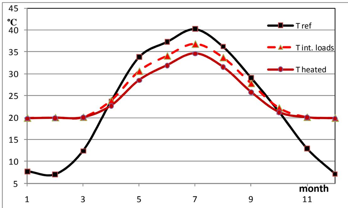
Figure 8.6 Monthly mean temperatures outdoors and in the building with and without heating system
