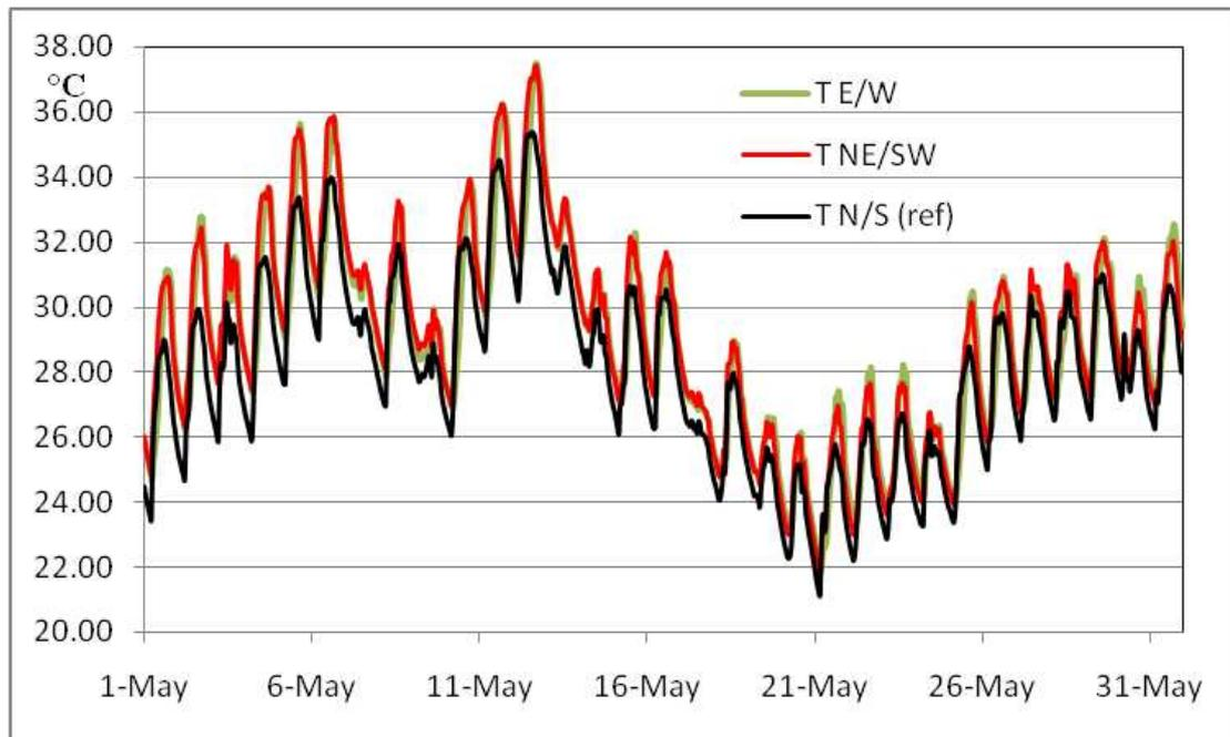
Figure 7.2 Temperatures in the building (with surrounding greenhouse) for different orientations
