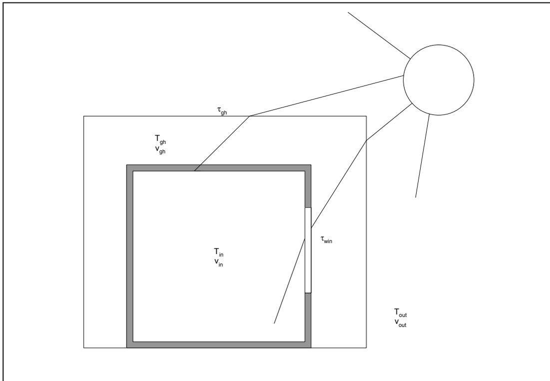
Figure 9.1 Schematic picture of the model of the building standing in the greenhouse.
