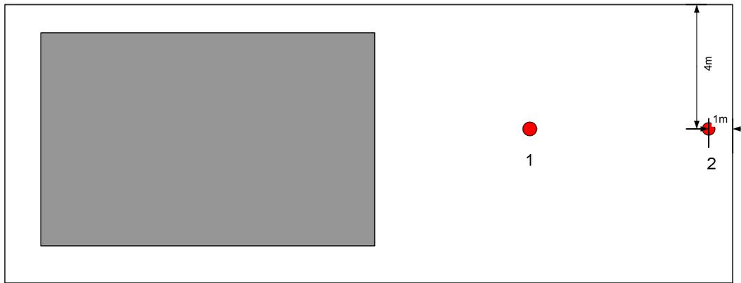
Figure 3.2 Placement of the loggers for measuring the climate in the volume of the greenhouse.
