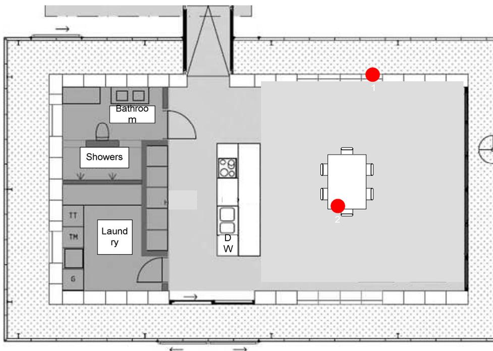
Figure 3.3 Measuring points for the climate in the building
