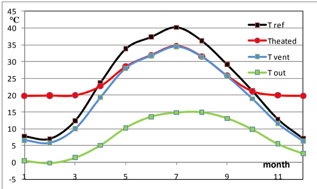
Figure 8.7 Effect of the ventilation on the monthly mean temperatures
