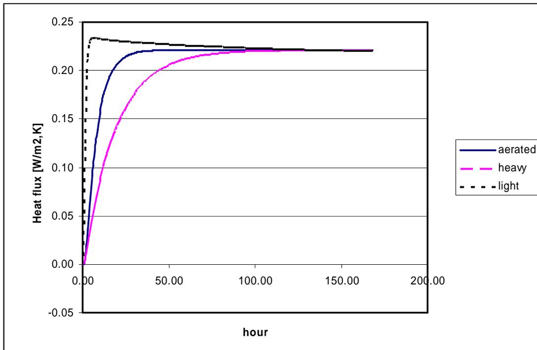
Figure 11.2 The thermal behavior of the walls when the thickness of the aerated concrete is reduced to 10cm and insulation is used to balance the U-value.
