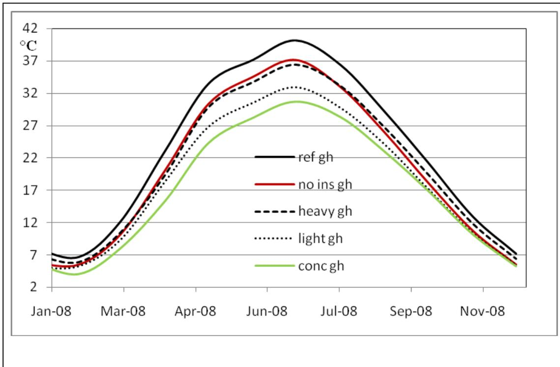
Figure 10.4 Indoor temperatures for the buildings in the greenhouse.
