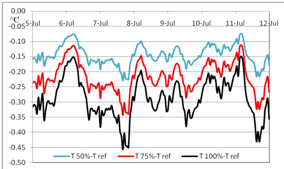
Figure 7.9 Difference in temperature between the reference case and the cases with screened roof during 7-13 July
