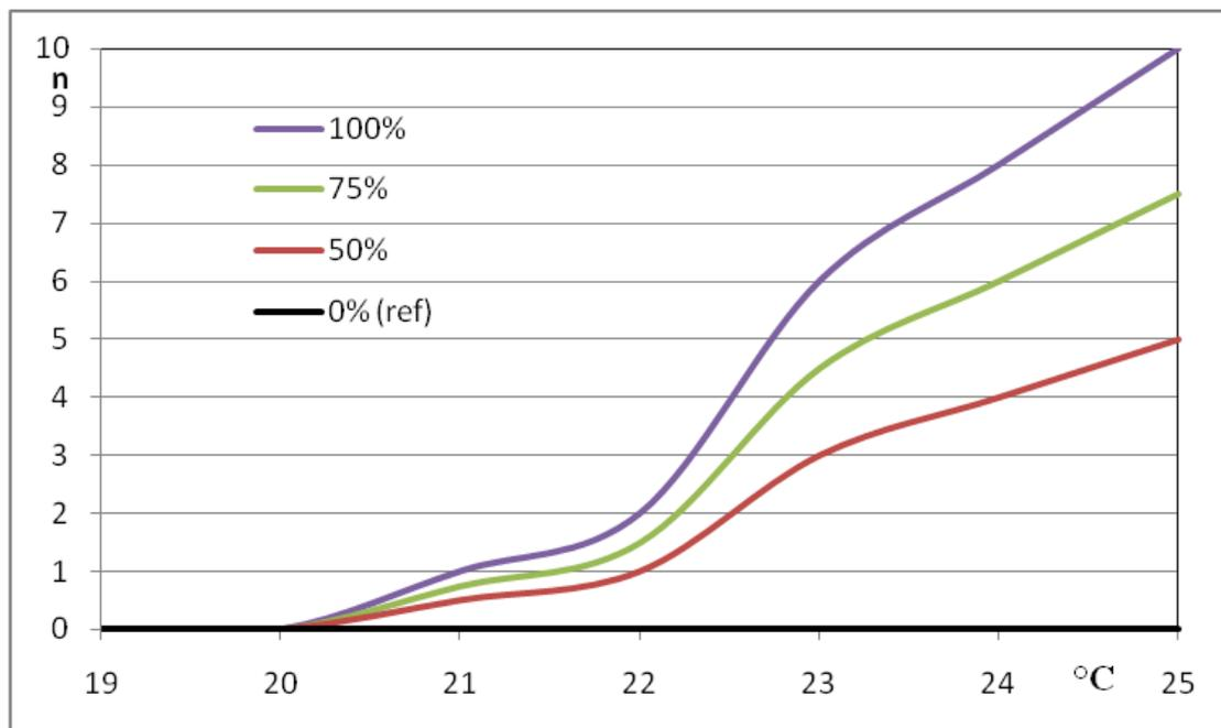
Figure 7.5 Air changes in the greenhouse due to temperature and degree of opening of the hatches
