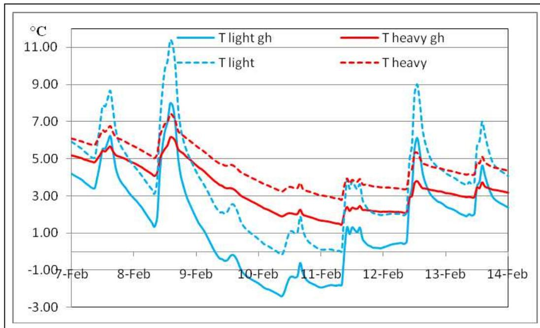
Figure 10.1 Temperatures in the building with and without greenhouse during the cold week. Designs with equal U-value.
