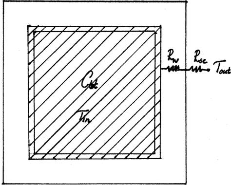
Figure 4.1  $C_{tot}$  and resistances for a wall calculated with Lumped System Analysis.
