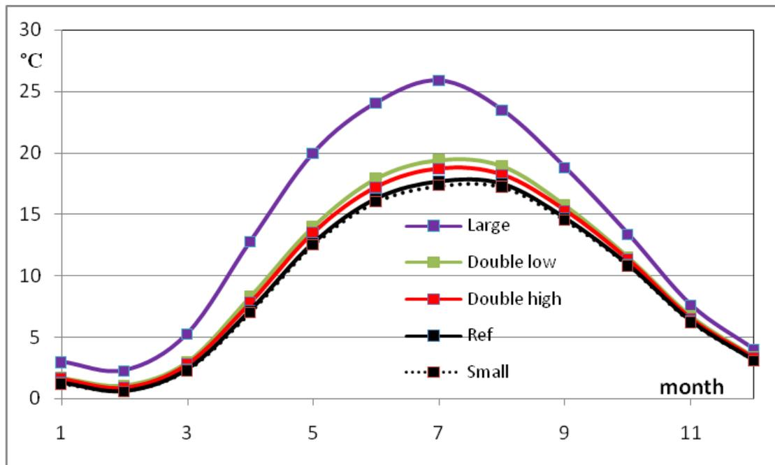
Figure 7.3 Monthly mean temperatures for the different sizes of the greenhouse.
