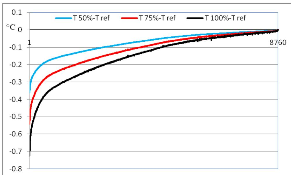
Figure 7.8 Difference in temperature between the reference case and the cases with screened roof
