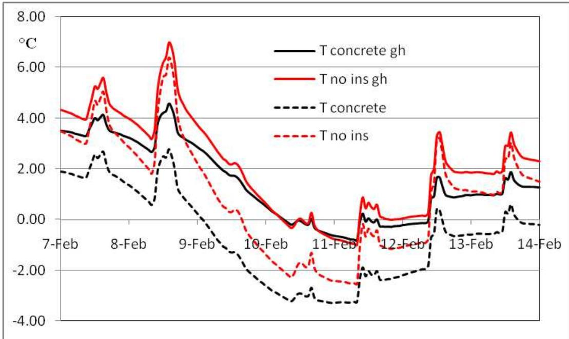
Figure 10.2 Temperatures in the building for changes in the original design, with and without the greenhouse during the cold week.
