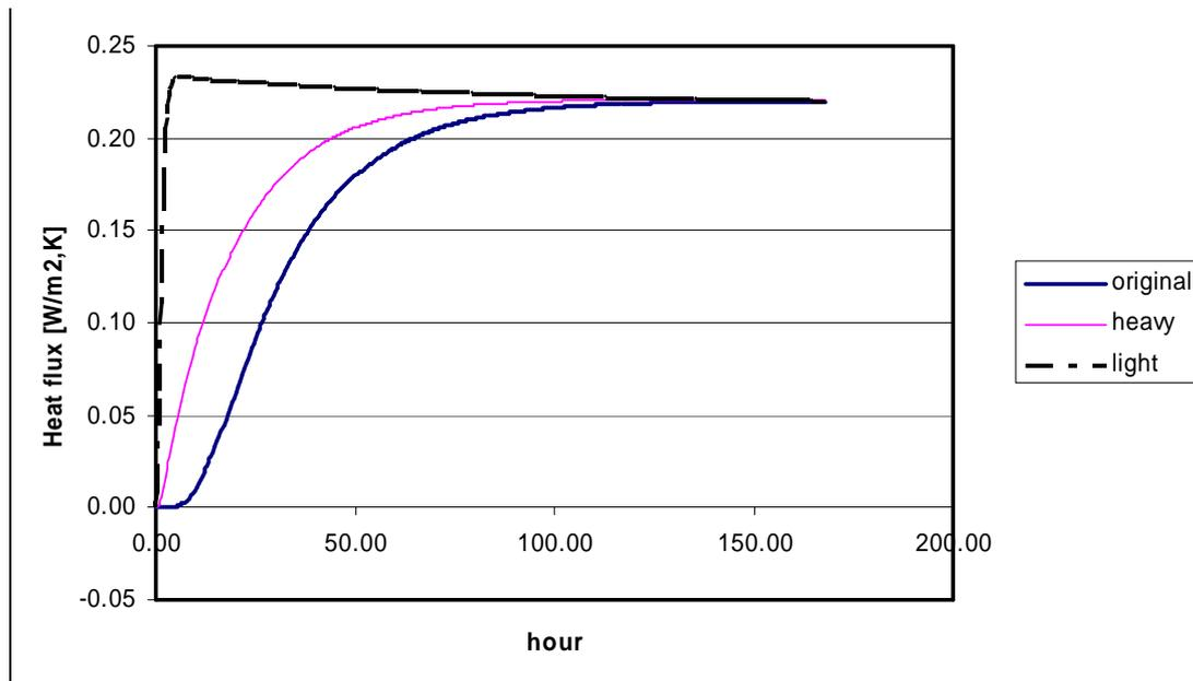
Figure 11.1 Thermal behavior of the three different wall constructions.
