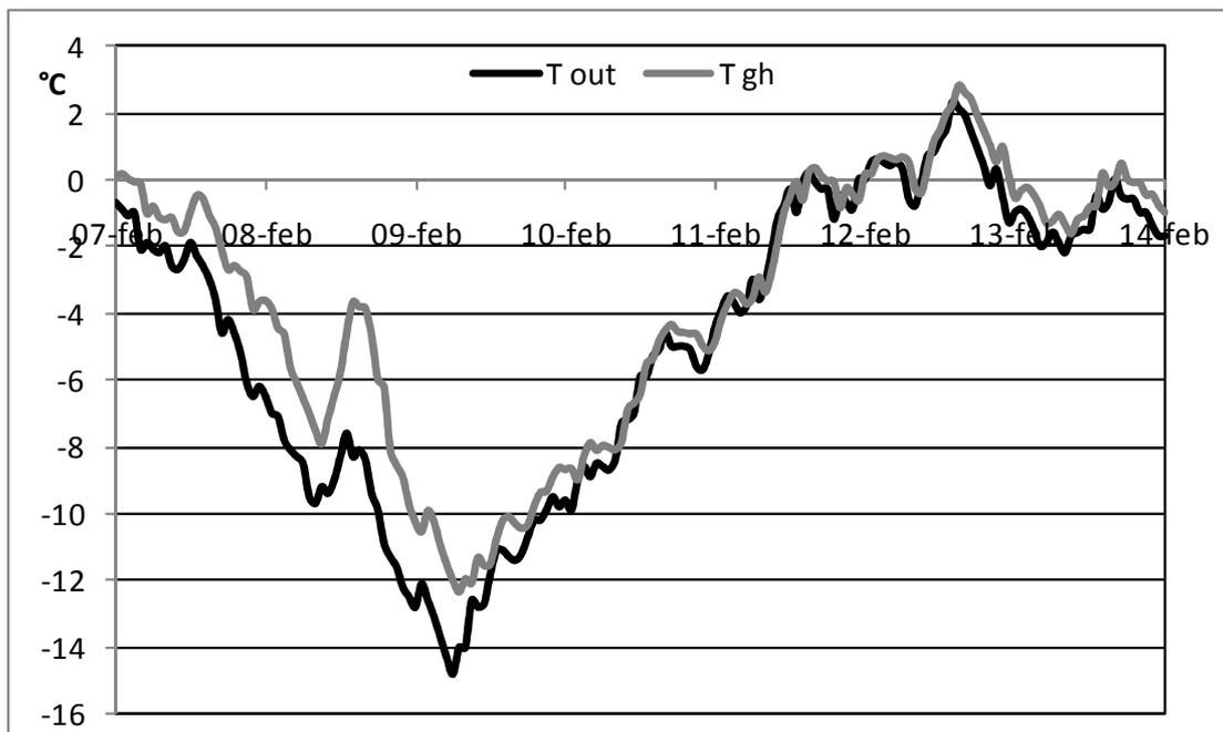
Figure 10.3 Temperatures in the building for changes in the original design, with and without the greenhouse during the cold week.
