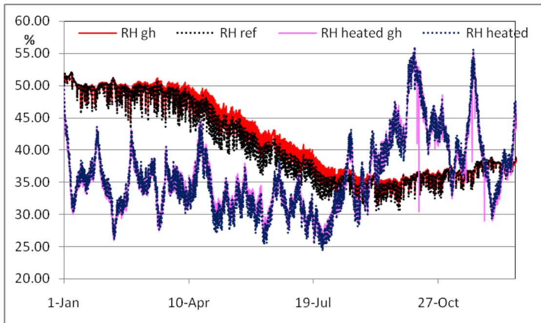
Figure 9.3 Relative humidity for the simulations of the building with and without greenhouse and with and without heating system.
