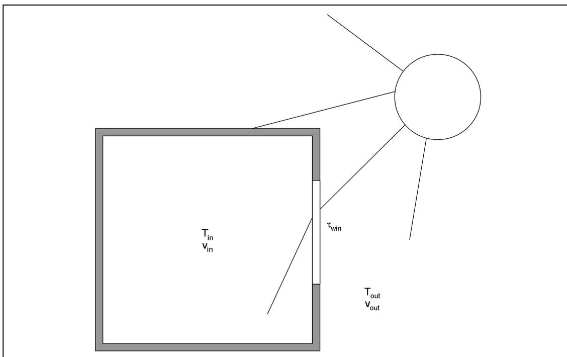
Figure 8.1 Schematic picture of the climate in the building. The indoor climate is affected by outdoor conditions and the buildings properties.
