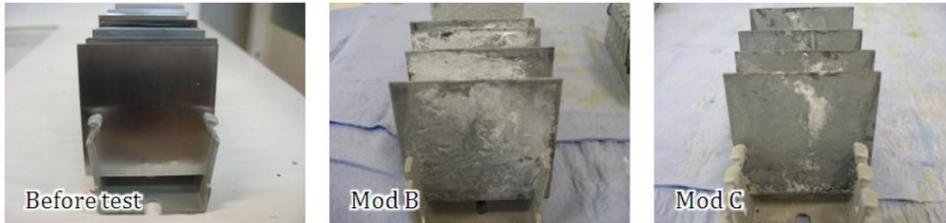
**Figure 12** Pictures of zinc coupons before and after test ISO 21207 method B Modification B (Mod B) and Modification C (Mod C).
