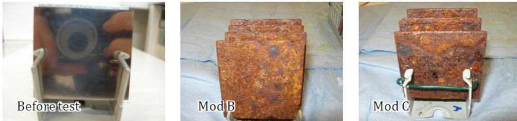
**Figure 8** Pictures before and after test ISO 21207 method B Modification B (Mod B) and Modification C (Mod C) of carbon steel coupons.
