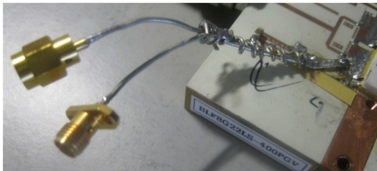
Figure 4.36 Picture of Probe used to measure Baseband Impedance
