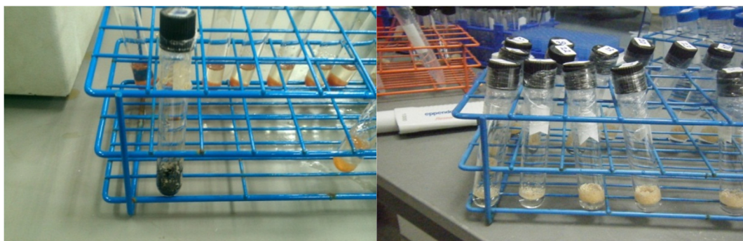
Figure 19 displays two typical experimental issues during this work. The sulfuric acid often evaporated causing the sample to burn and this is illustrated in the image to the left. The substrate attached to the sides after the dilute acid was added to the sample and this is shown in the picture to the right.
