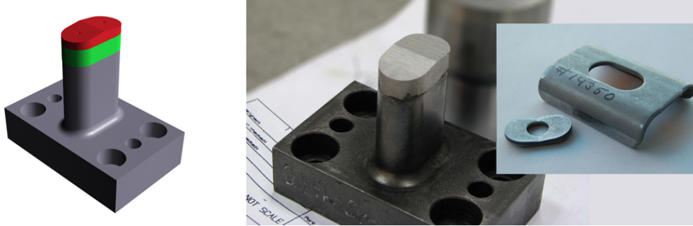
Figure 4.3: Left: A CAD drawing of the punching die. Right: The final die obtained by deposition high grade steel onto a mild steel die shoe. The image also shows the punched part with the removed piece lying aside.
