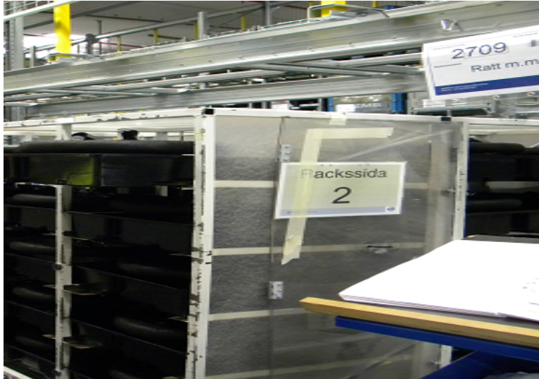
Figure.4.6 Sequencing rack loaded with materials
