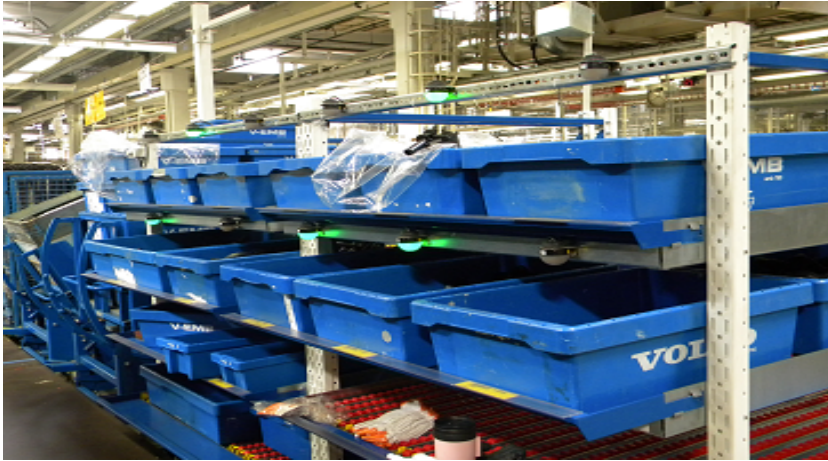
Figure.4.8 Pick to light system for components with many variants
