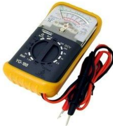
Figure 7: Analog multimeter used in our experiment.
