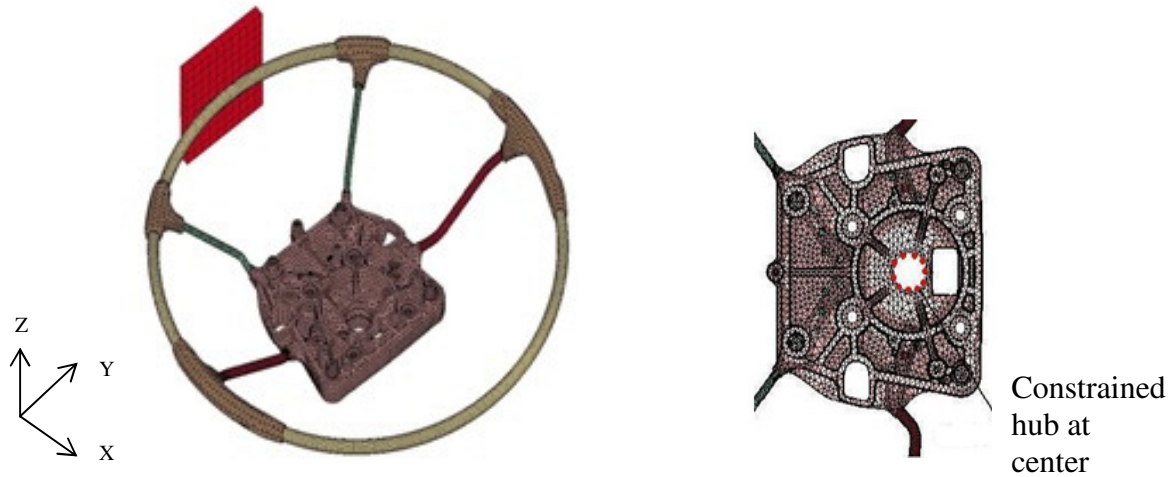
(a) Steel plate impact with the steering wheel
