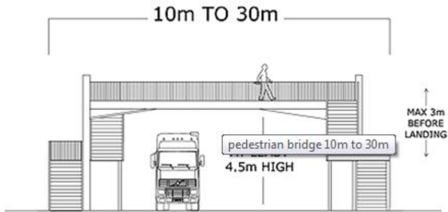
Figure 4.22 A typical pedestrian bridge with minimum headroom and span range [18].
