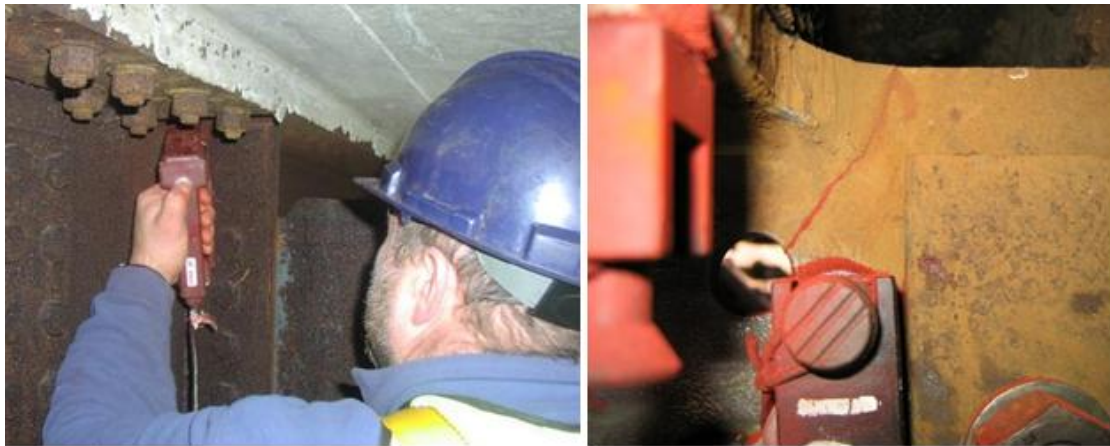
Figure 3.3 Operation of MPI test [23].
