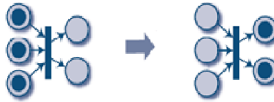
Figure 3. Transition of tokens over an activity in a Petri net (Wynn, 2007, p.44)
