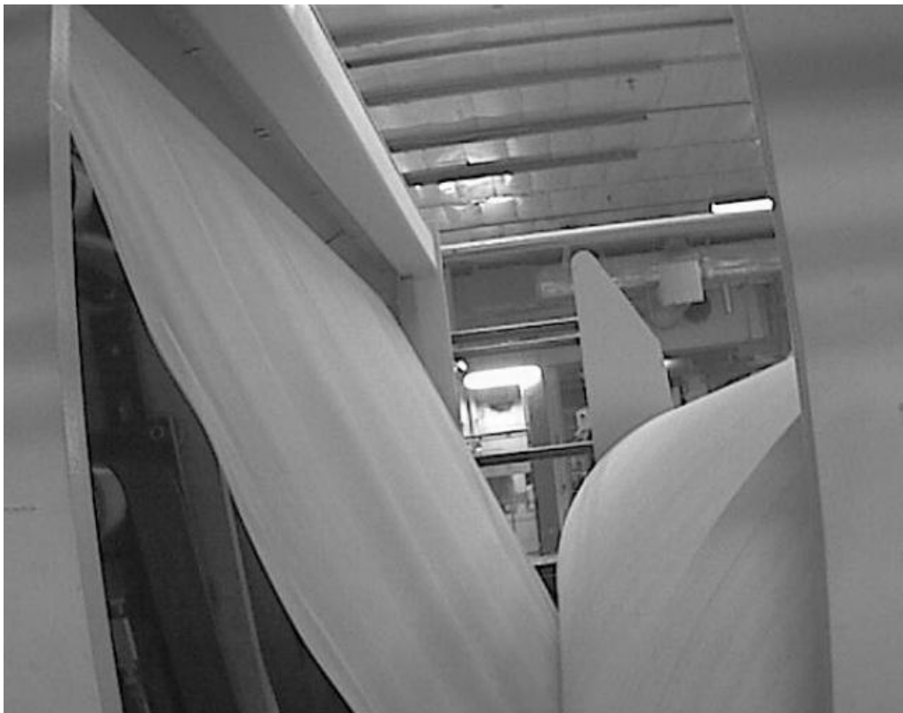
Figure 19 Web-flutter during unwinding on Driver side, Stand 3.
