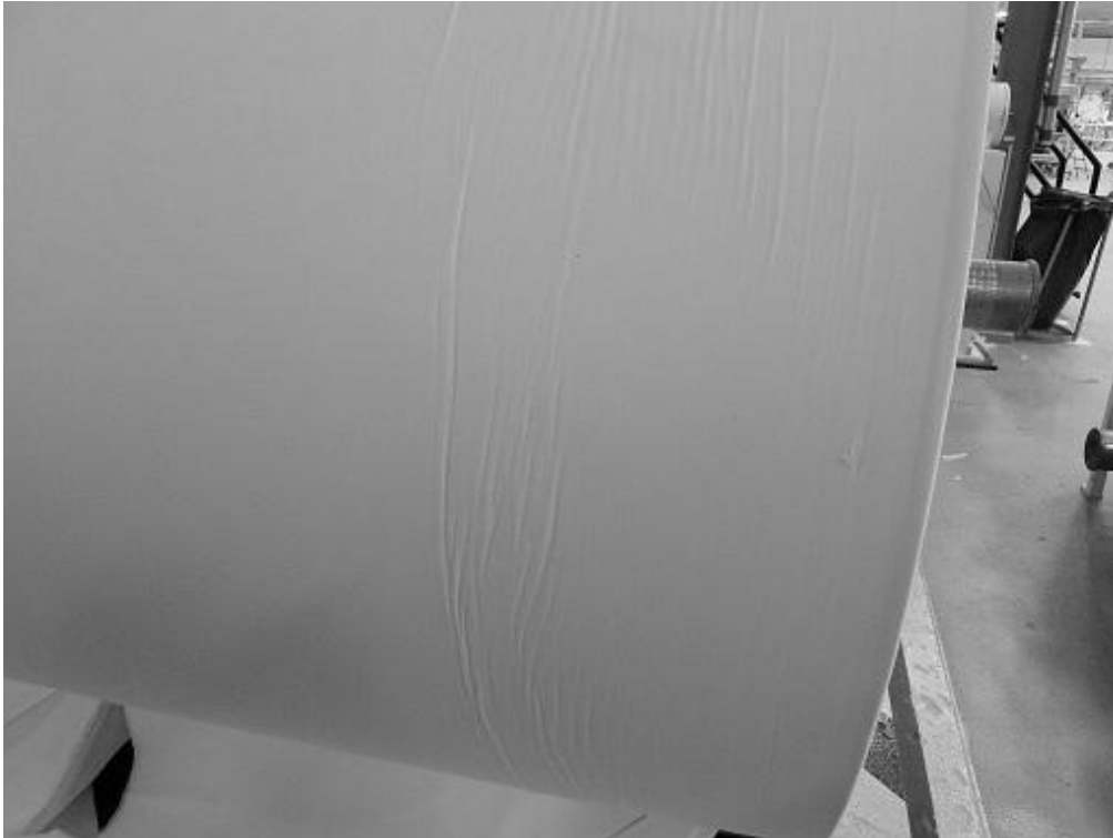
Figure 3. Visible wrinkles on a mother reel.
