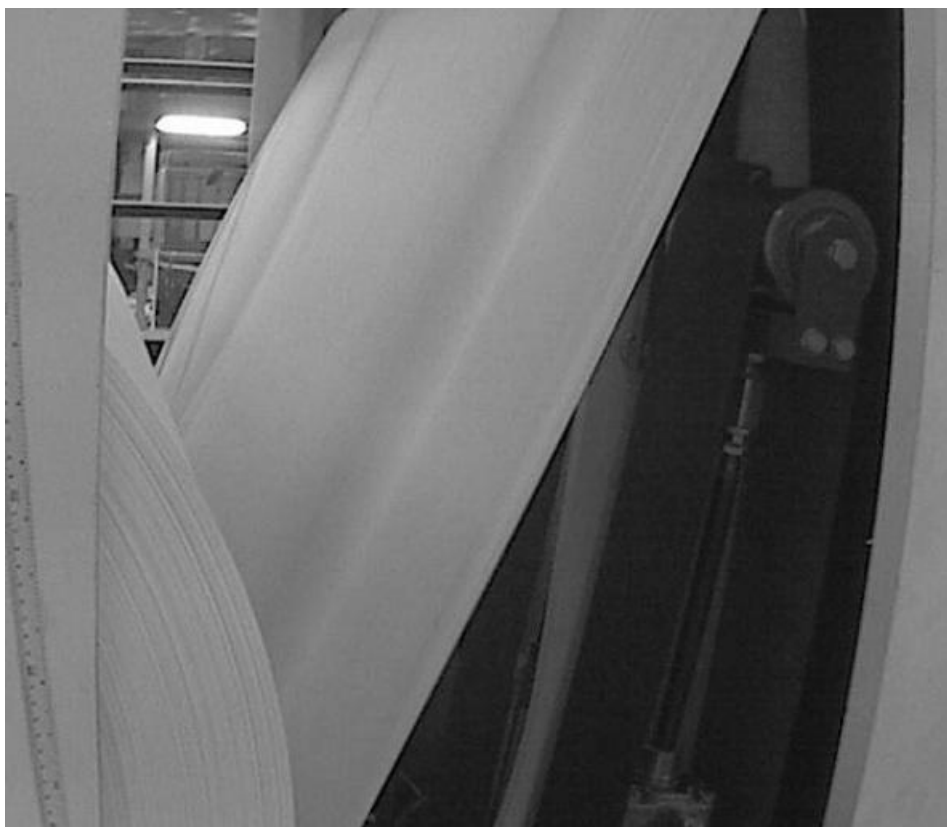
Figure 2. Visual slackness and tautness in the web (baggy web) during unwinding.
