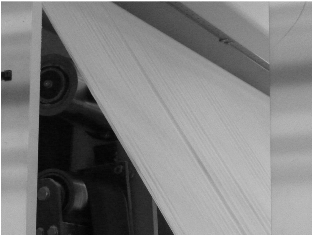
Figure 21 Wrinkles in web while running during unwinding.
