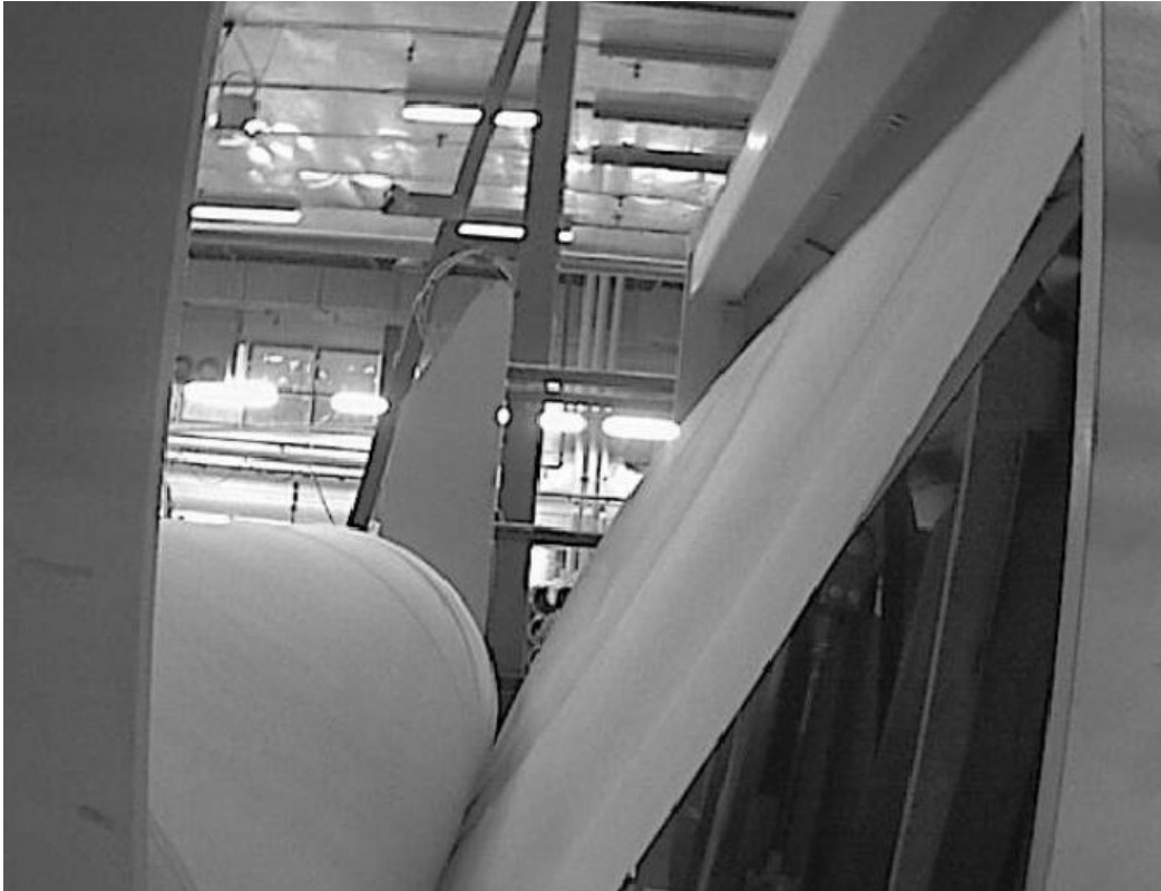
Figure 20 Web-flutter during unwinding on Operator side, Stand 4.
