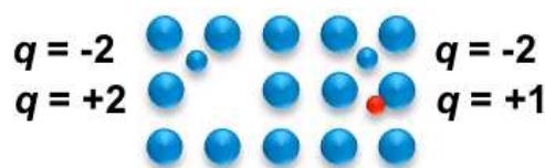
Figure 4.6: Schematic illustration of acceptor dopants trapping oxygen vacancies (left) and protons (right).
