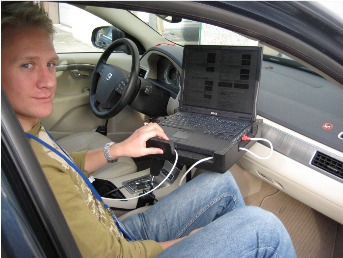
Figure B.3 Jonas Östh with laptop running control and logging software in the test vehicle.
