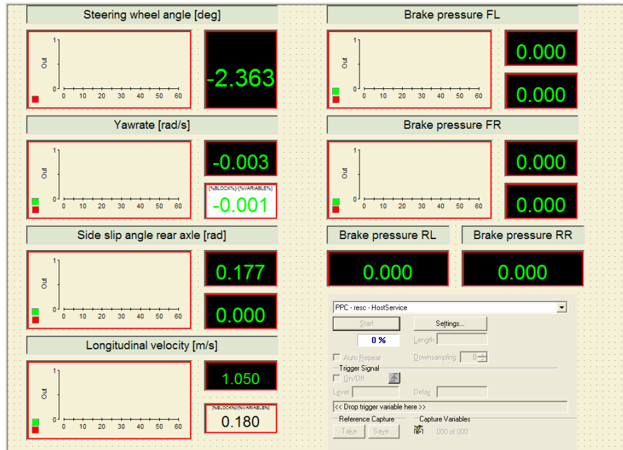
Figure 4.7 The monitor and logging interface developed in Dspace ControlDesk.
