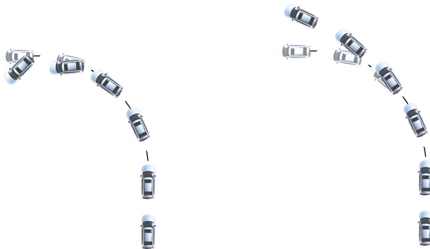
Figure 1.2a Oversteer situation, vehicle yaws too much compared with driver intent.
