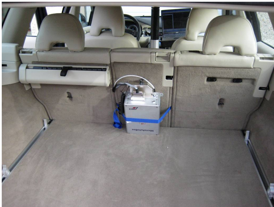
Figure B.2 Dspace MicroAutoBox running controller model placed in the luggage compartment of the test vehicle.
