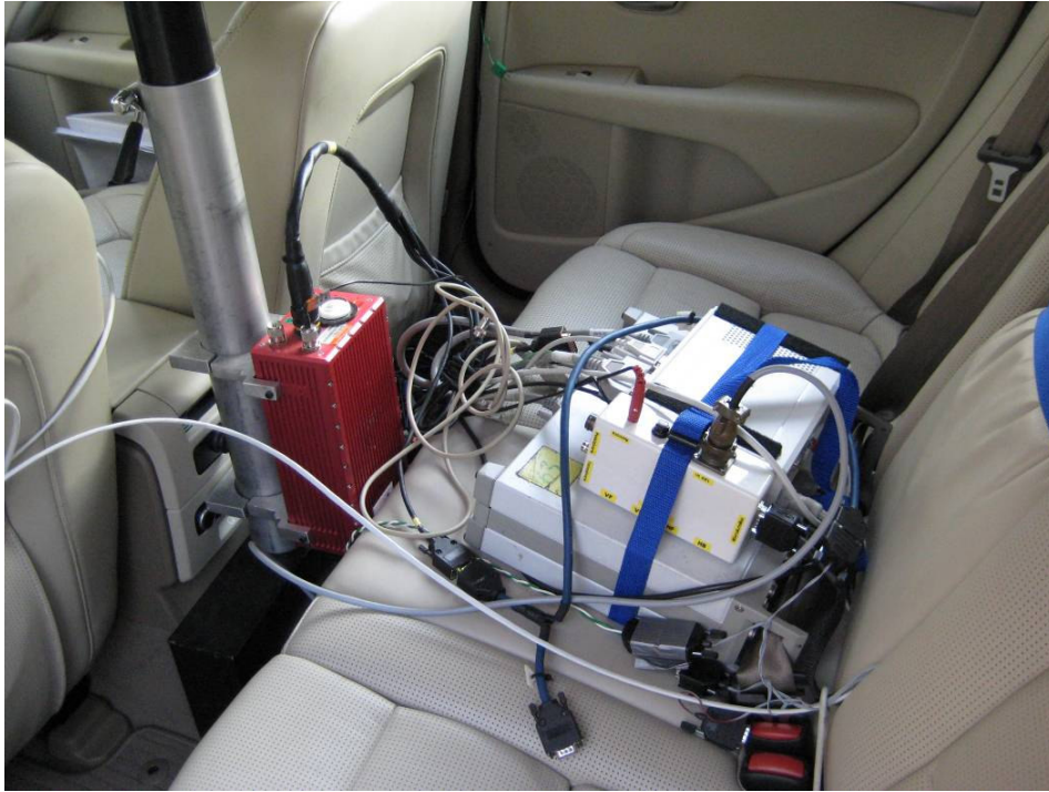
Figure B.1 OXTS RT3000 GyroScope mounted between roof and floor and Data Acquisition System placement in the back seat of the test vehicle.
