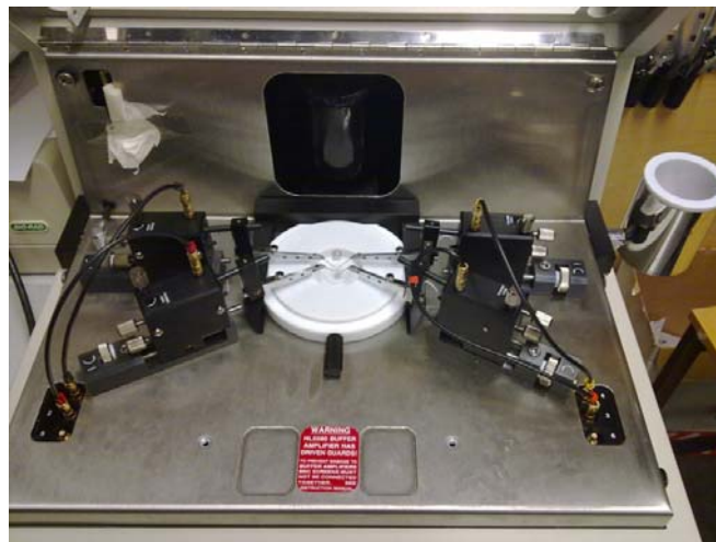
Fig. 16 The Hall Effect machine on 6 th floor
