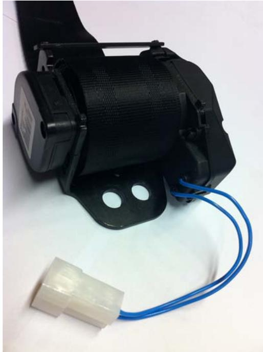
Figure 4.4: Truck belt retractor used for the prototype
