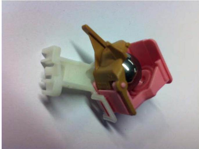
Figure 1.1: Mechanical car sensor
