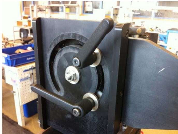
Figure 4.9: Tilt adjustment for tilt test bench
