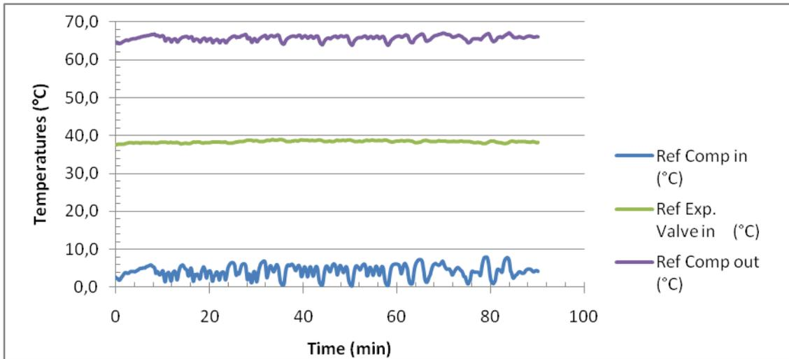
Figure 6.20: Temperatures given by Climacheck sensors for the 90 minutes selected sample
