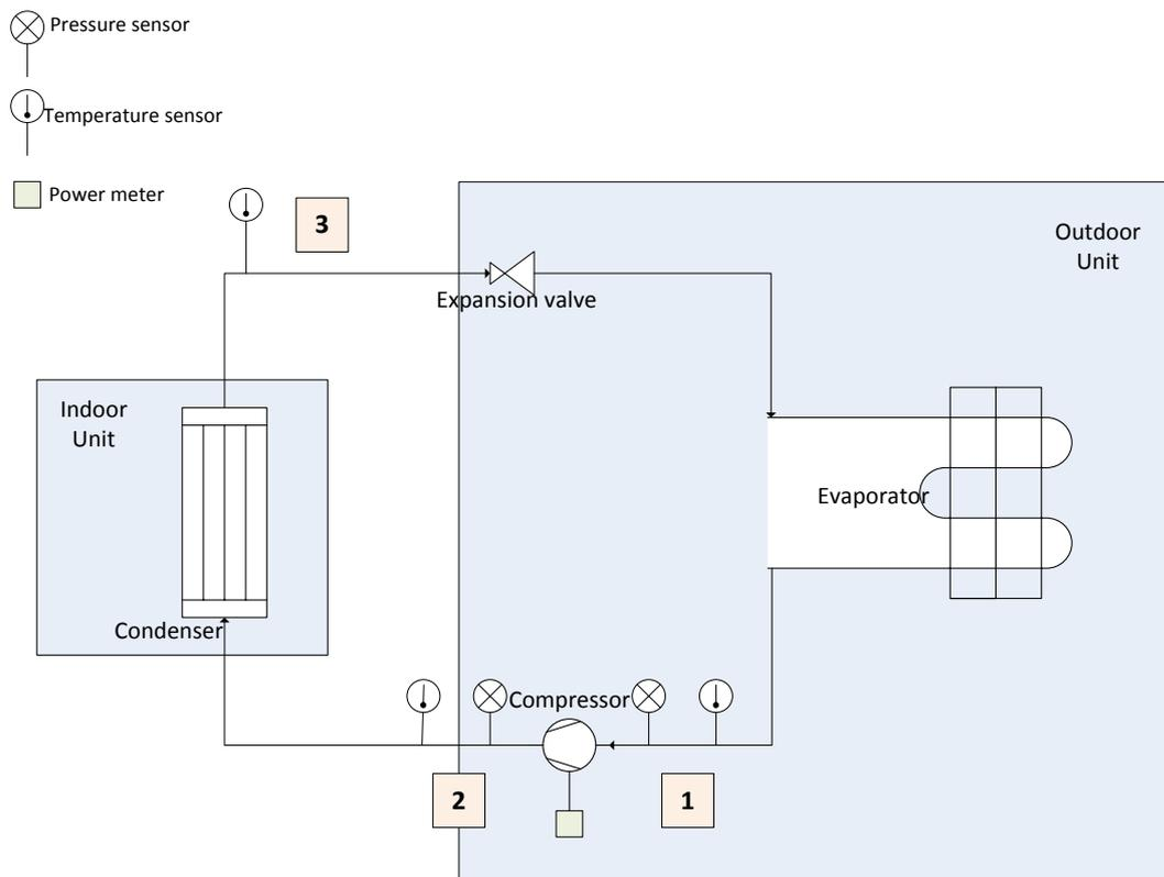
*Figure 3.8: Instrument setup for the Climacheck Method*
