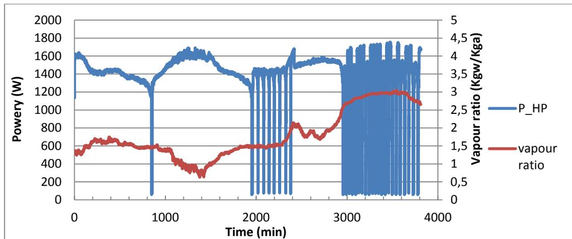
Figure 6.2: Influence of vapour ratio to heat pump performance
