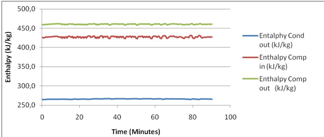
Figure 6.19: Enthalpies obtained with Climacheck sensors and software for the 90 minutes selected sample
