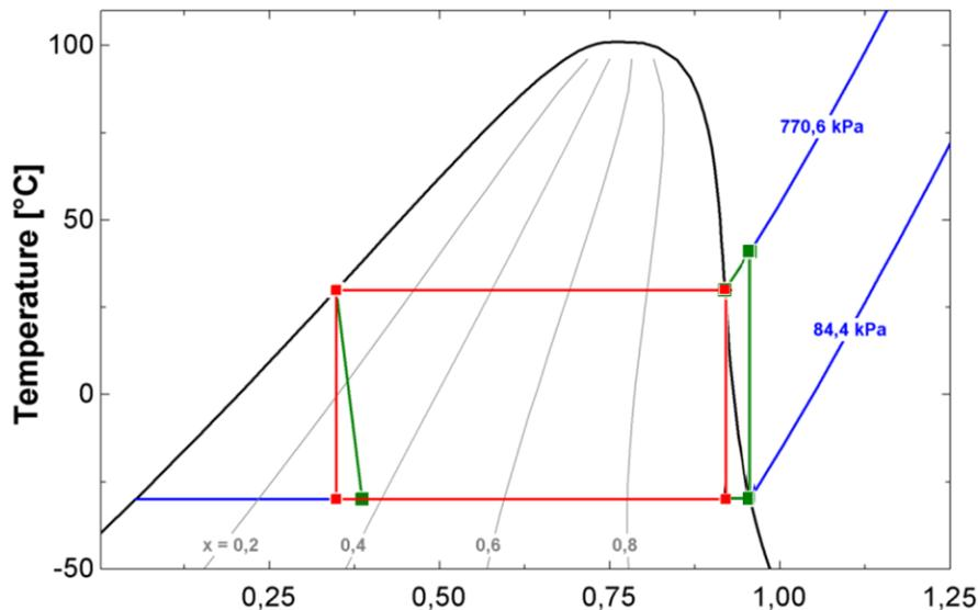
Figure 3.4: A Carnot process (red lines) overlaid a basic vapour compression process (green lines) on a T-s diagram
