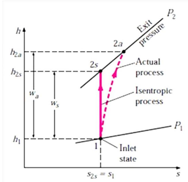
Figure 6.18 : Diagram  $h$ - $s$  showing the difference between the actual compression process and the isentropic one (General case)
