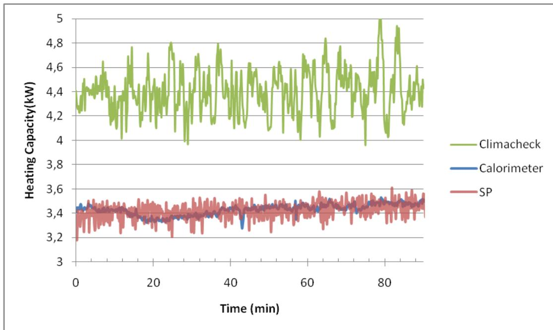
Figure 6.16: Heating Capacity calculated from Calorimeter, SP and Climacheck Method during the same testing period
