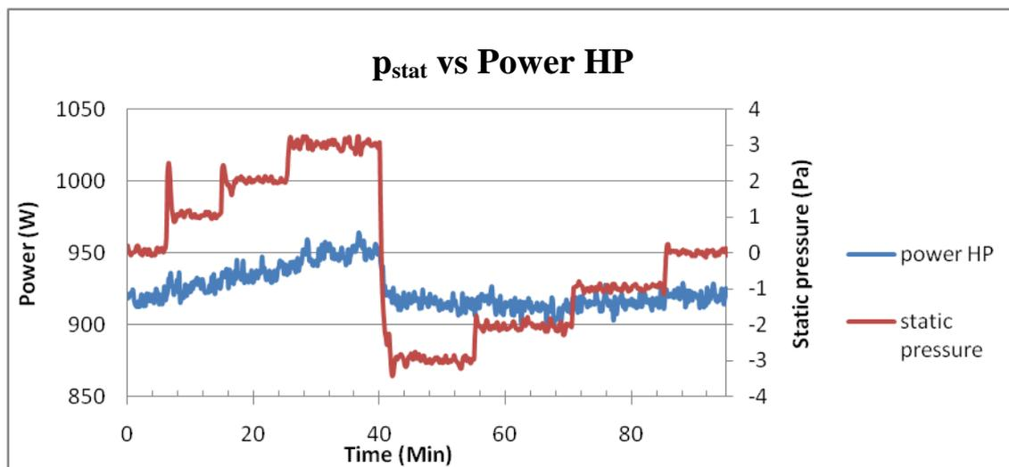
Figure 6.10: Static pressure vs Power consumption of heat pump
