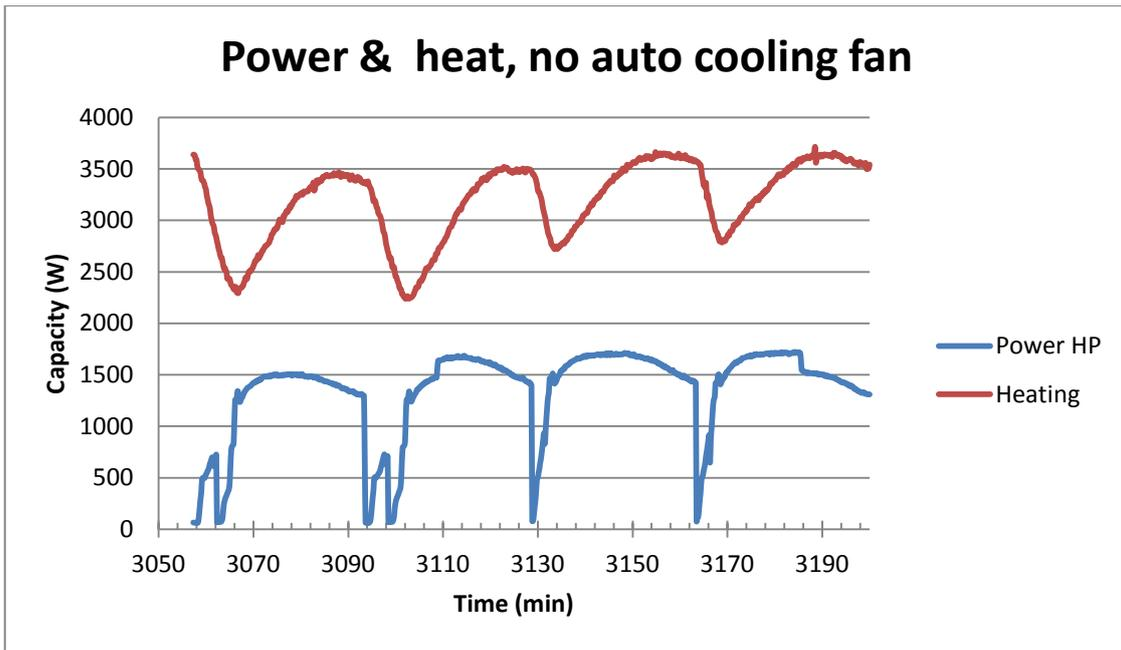
Figure 6.7: Power & heat, no auto cooling fan
