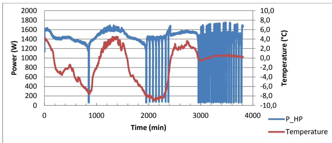
Figure 6.3: Influence of air temperature to heat pump performance
