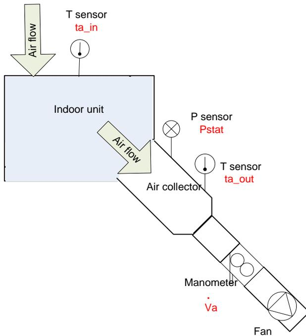
Figure 3.6: Equipment setup for the SP Method
