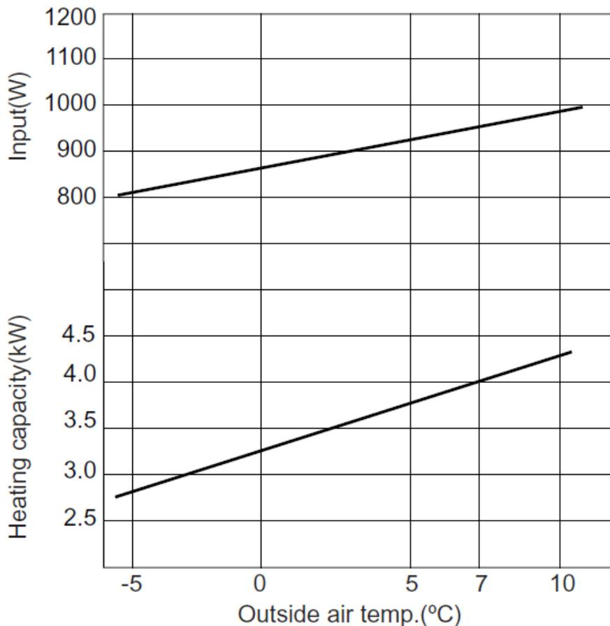
*Figure 4.4: Performance of BOSCH 6.0AA Heat Pump in heating mode with 20°C indoor temperature and variable outdoor temperature*
