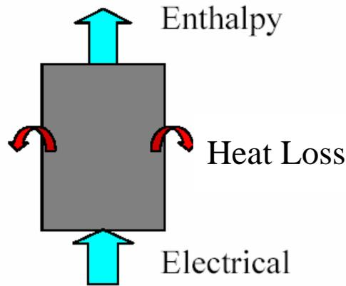
Figure 3.12: Energy flows through the compressor
