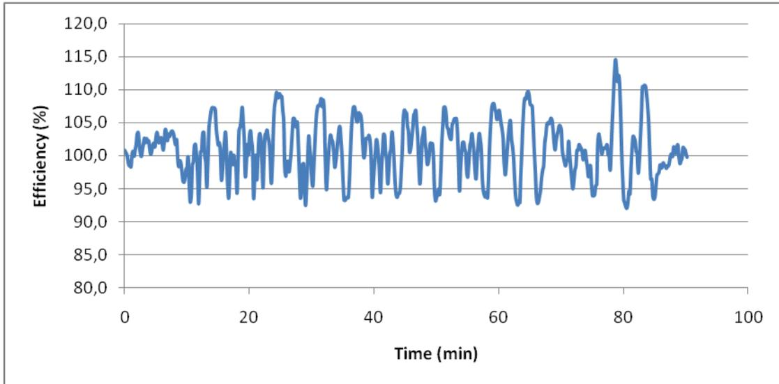
Figure 6.17 : Isentropic efficiency observed by Climacheck
