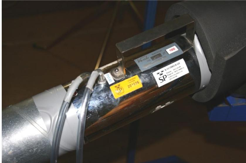
Figure 4.14: Air flow meter used for the SP Method
