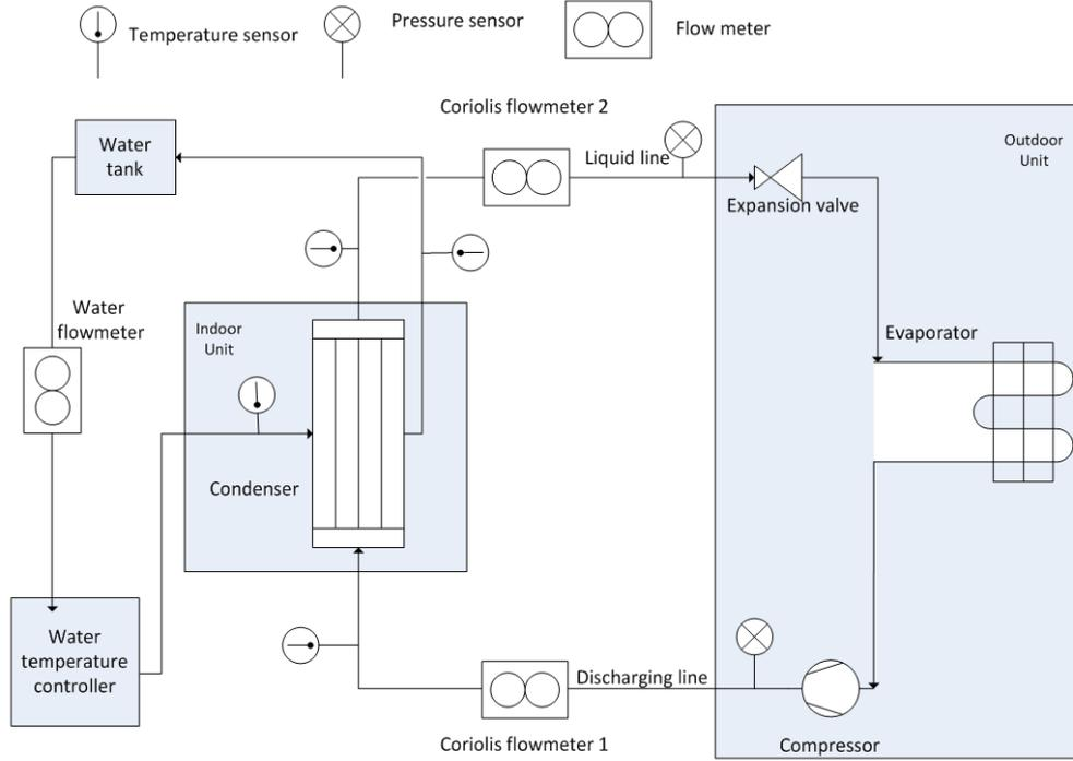
Figure 3.13: Instrument setup for refrigerant enthalpy method
