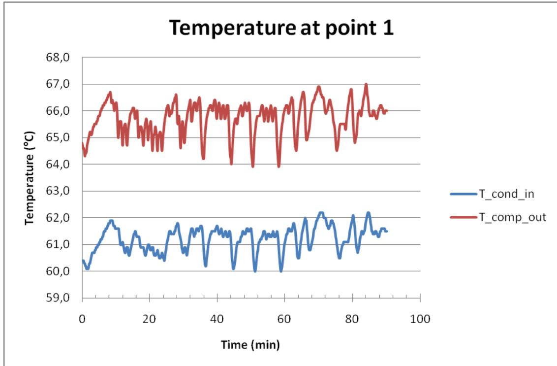
Figure 6.15: Temperatures measured at the condenser inlet and the compressor outlet
