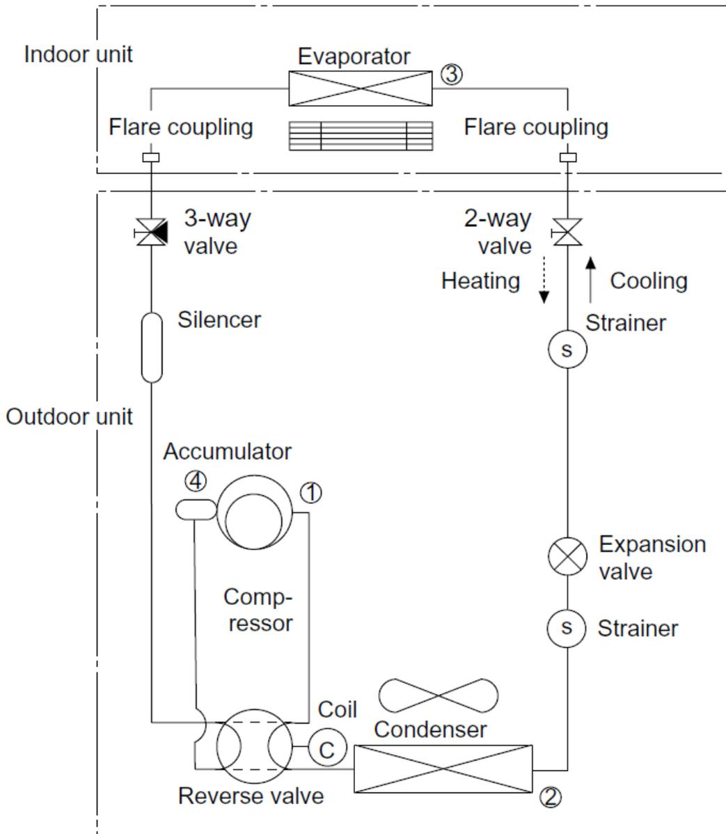
Figure 4.2: Refrigerant cycle schematic diagram of the tested unit
