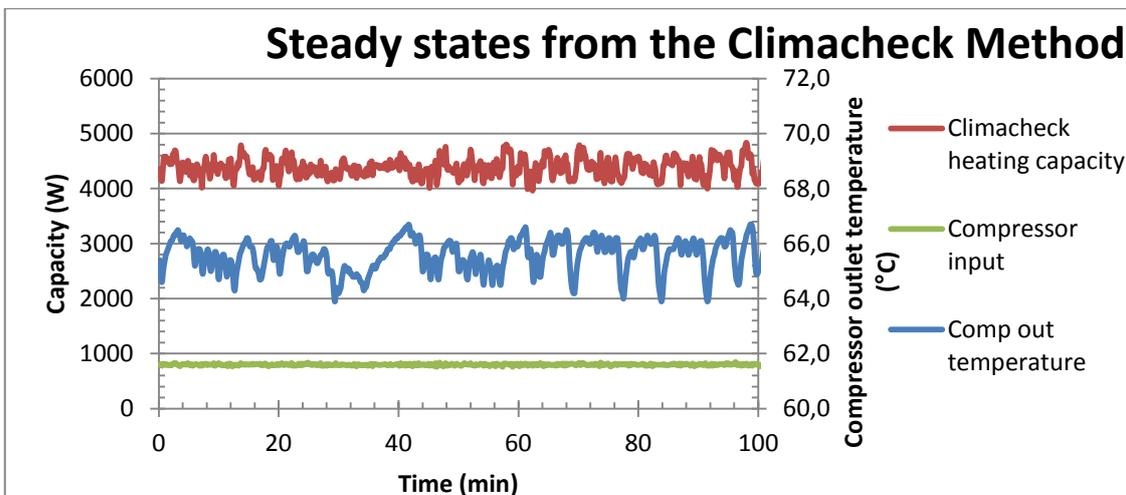
Figure 5.9: Steady state parameters from the Climacheck Method
