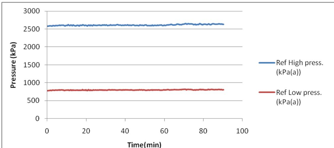
Figure 6.21: Pressures given by Climacheck sensors for the 90 minutes selected sample
