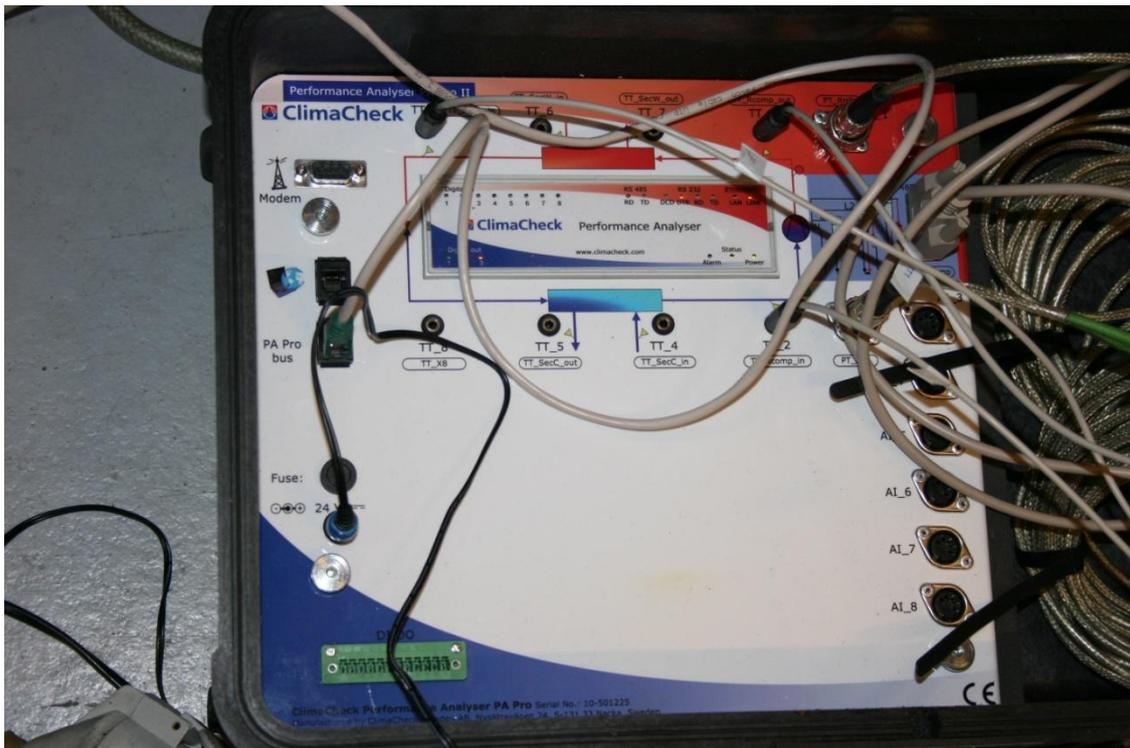
*Figure 3.10: Climacheck data logger with the sensors inserted*
