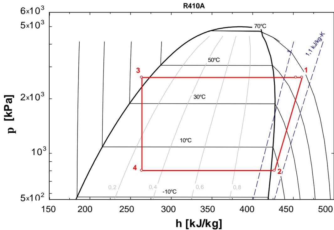
Figure 6.22: *p-h* diagram of the cycle at the studied point with Climacheck data plotted with the software 'Engineering Equation Solver'
