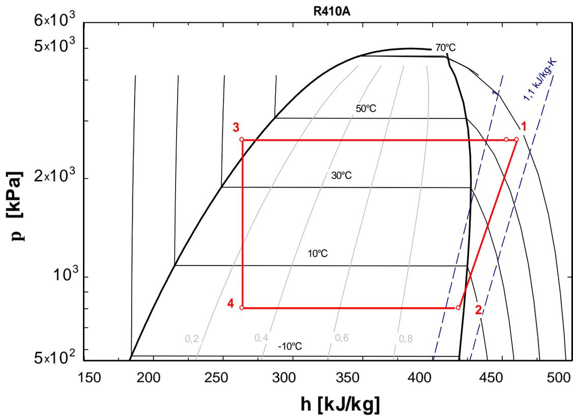
Figure 6.23 P-h diagram of the cycle at the studied point with assumption of Table 6.5 plotted with the software 'Engineering Equation Solver'
