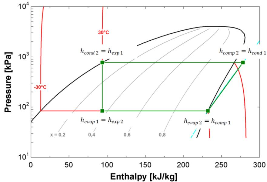
Figure 3.2: A basic vapour compression process illustrated on a p-h diagram
