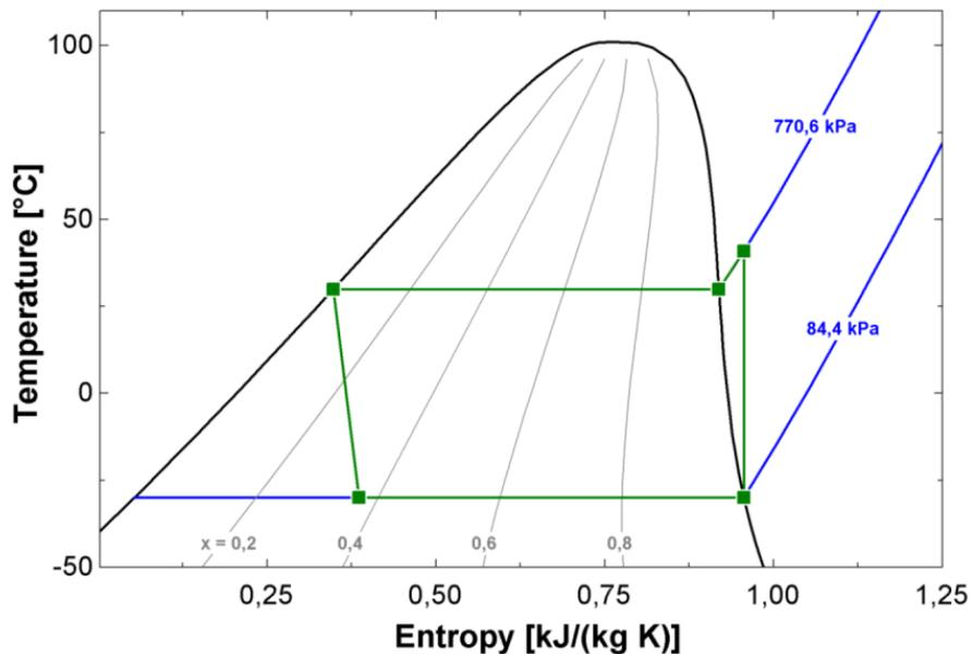
Figure 3.3: A basic vapour compression process illustrated on a T-s diagram
