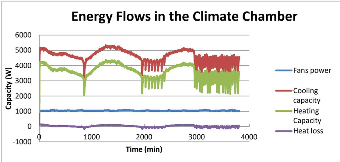
Figure 5.3: Energy Flows in the Climate Chamber
