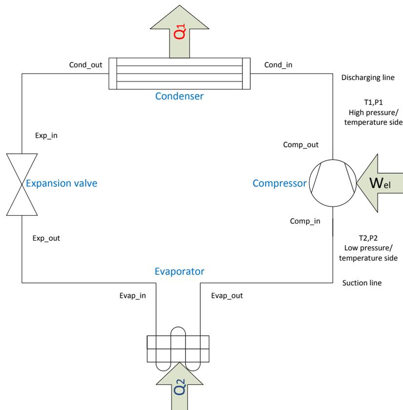
Figure 3.1: Principle scheme of heat pump
