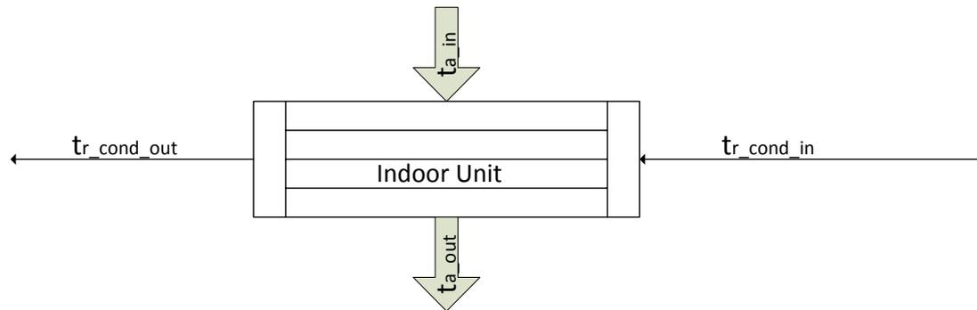
Figure 6.12: Temperature change through the indoor unit
