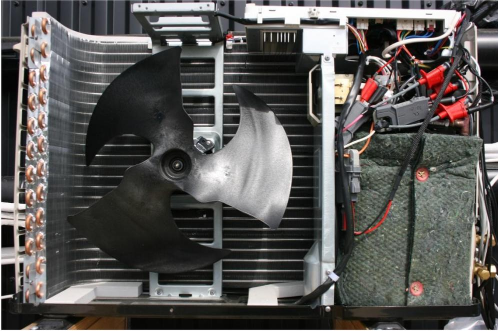
*Figure 4.15: Current and voltage clamps in the outdoor unit (the Climacheck Method)*
