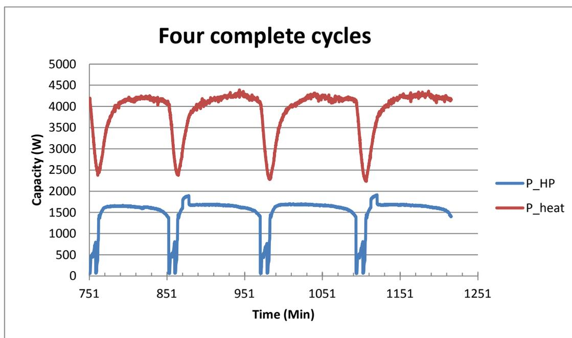
Figure 6.1: Four complete cycles with defrosting resulting from measurements by the Calorimeter Method
