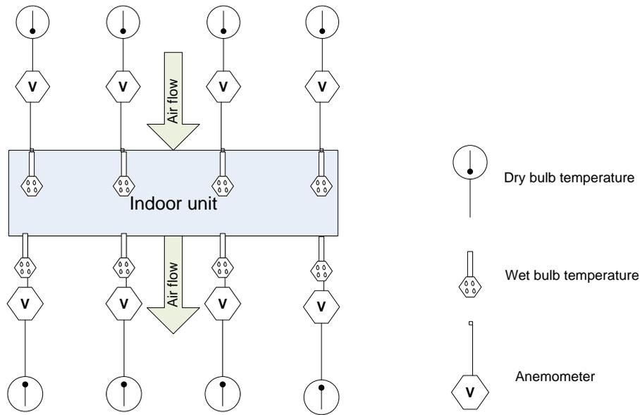
Figure 3.7: Instrument setup for Tokyo Gas Method
