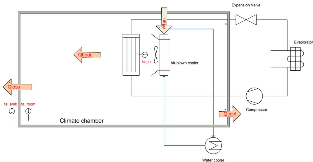
Figure 3.14: Equipment setup and energy flow of indoor compartment for the Calorimeter Method
