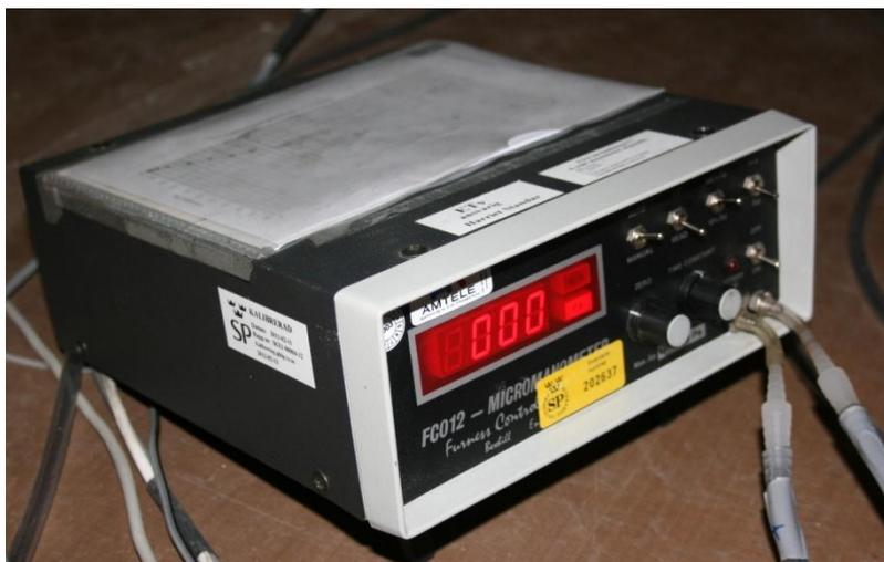
Figure 4.13: Manometer Furness FCO12 used for the SP method
