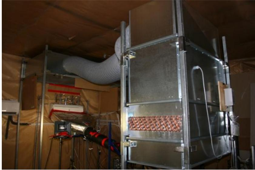
*Figure 4.8: The Calorimeter Method set up with cooling fan above the indoor unit on the left-side of the picture and the air-water heat exchanger on the right-side*
