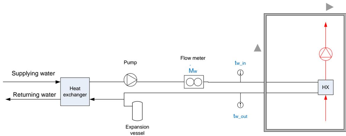
Figure 4.5: Cooling device sketch
