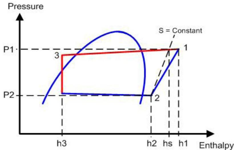
Figure 3.11: Refrigerant state with the corresponding points in p-h diagram
