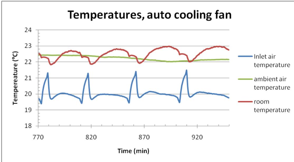
Figure 6.8: Measured temperatures, with auto cooling fan
