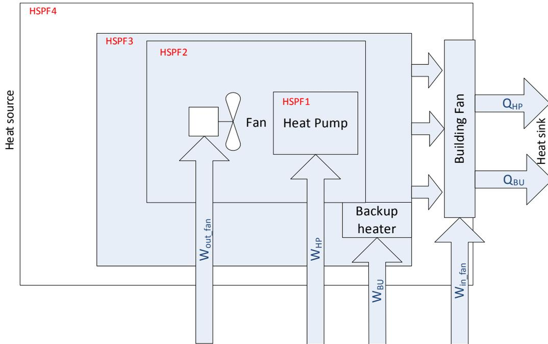
Figure 3.5: System boundaries for heat pump in heating operation
