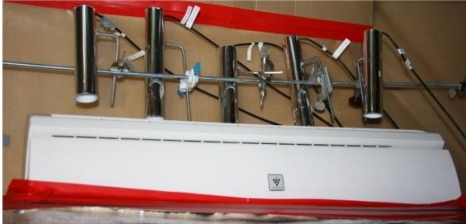
Figure 4.11: Temperature sensors at the air inlet of the indoor unit (the Calorimeter Method and the SP Method)
