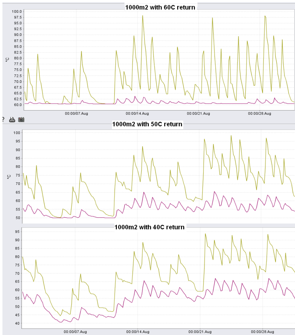
Figure 46 - Top and middle storage tank temperatures at varying network return temperatures
