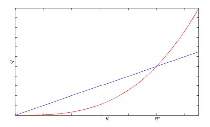
Fig 1. The radial dependence of heating and heat loss for the spherical discharge volume. Red curve is heating and blue curve is heat loss.
