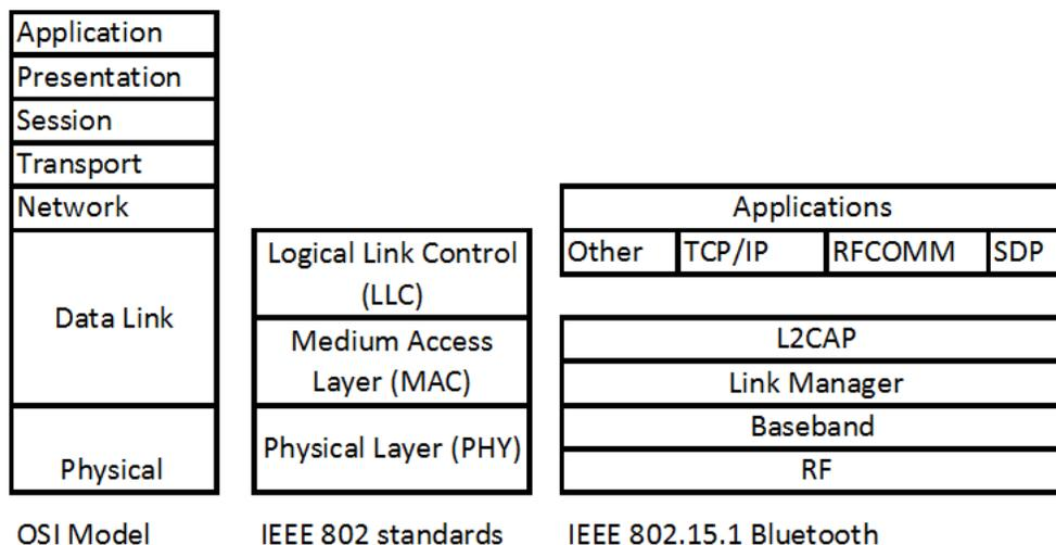
Figure 2.4: OSI reference Model, IEEE 802 family of standards and Bluetooth stack
