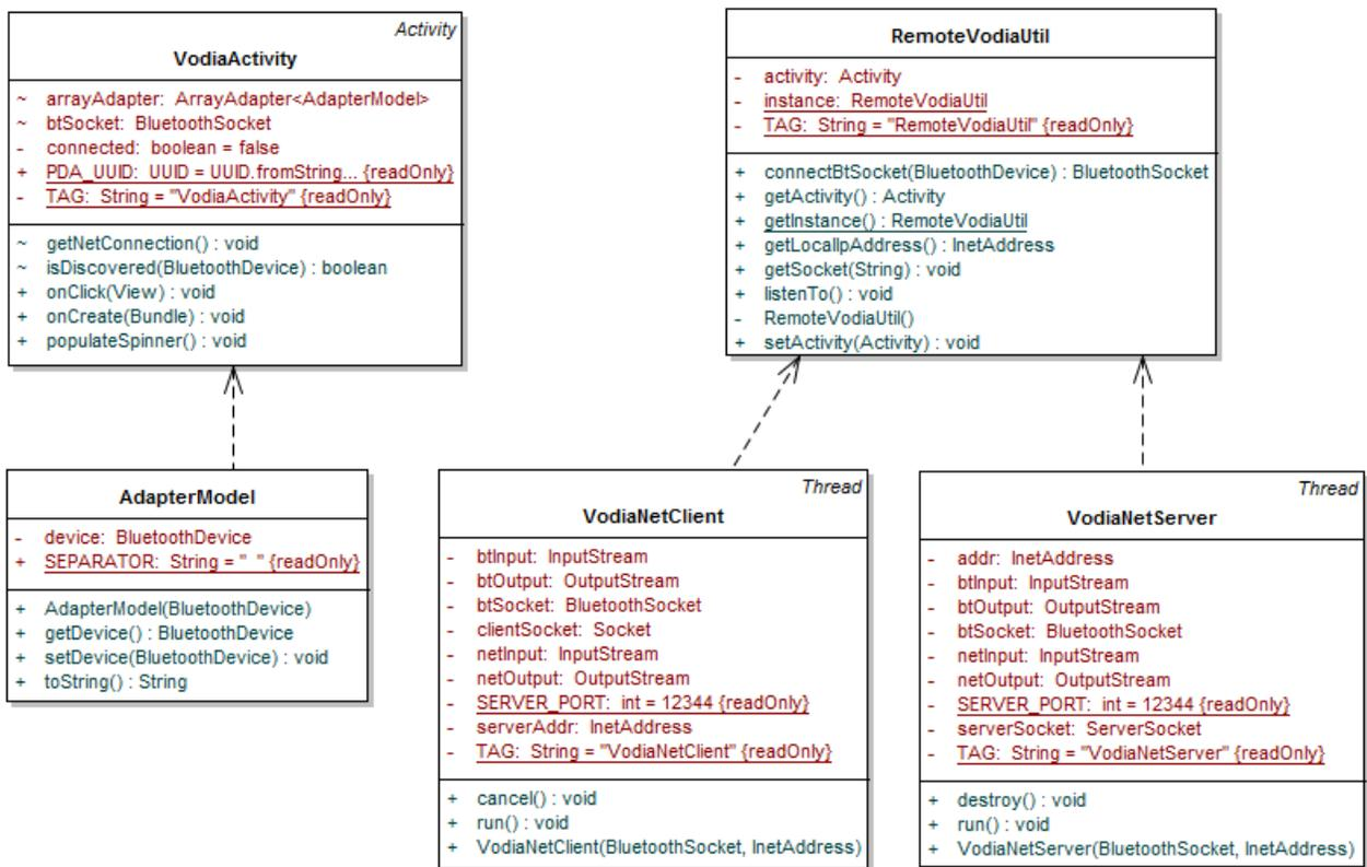
Figure 4.7: The class diagram of the Android application
