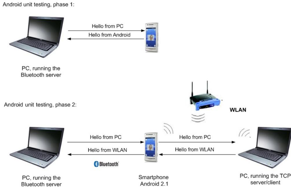
Figure 6.1: Hardware setup used for testing the Bluetooth and TCP server/client functionality on the smartphone
