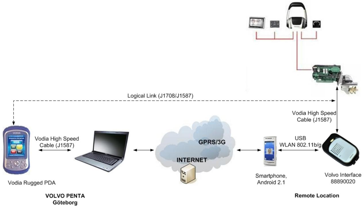
Figure 4.2: Possible architecture for the remote diagnostic system's prototype
