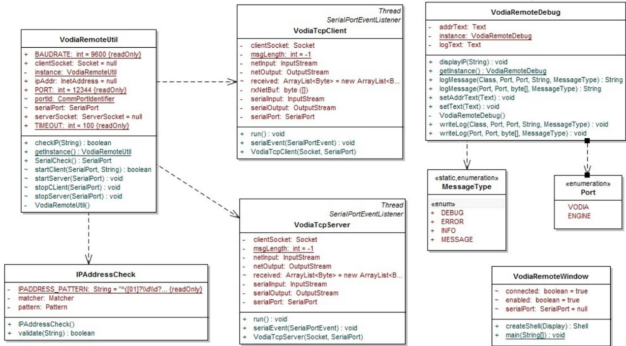
Figure 4.9: The class diagram of the “Remote Diagnostic Tool” application
