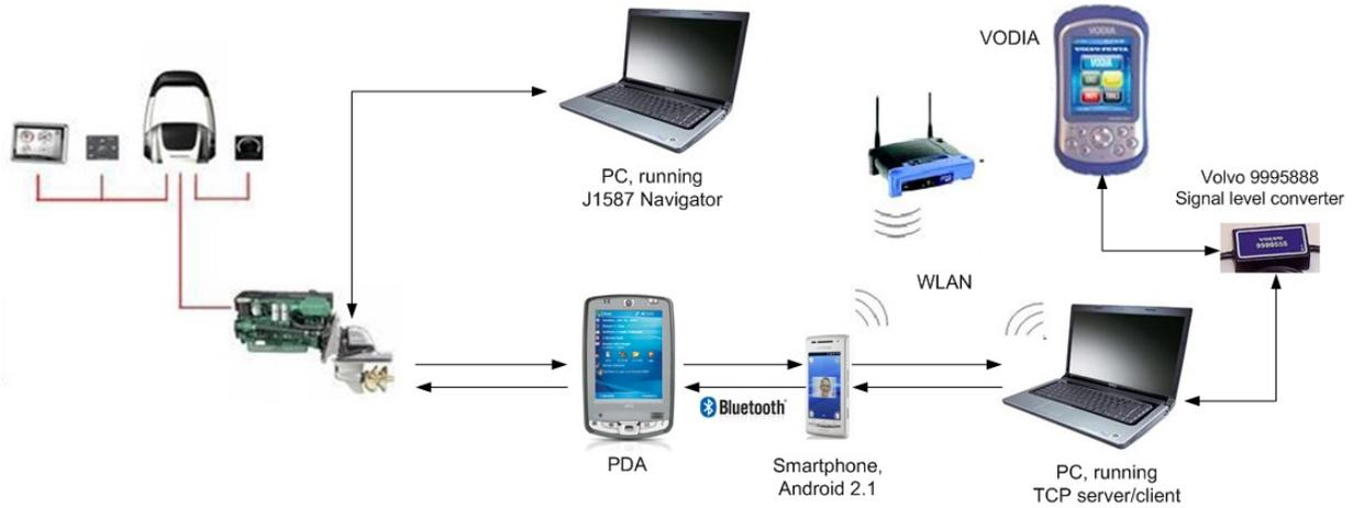
Figure 6.5: Hardware setup used for prototype's testing
