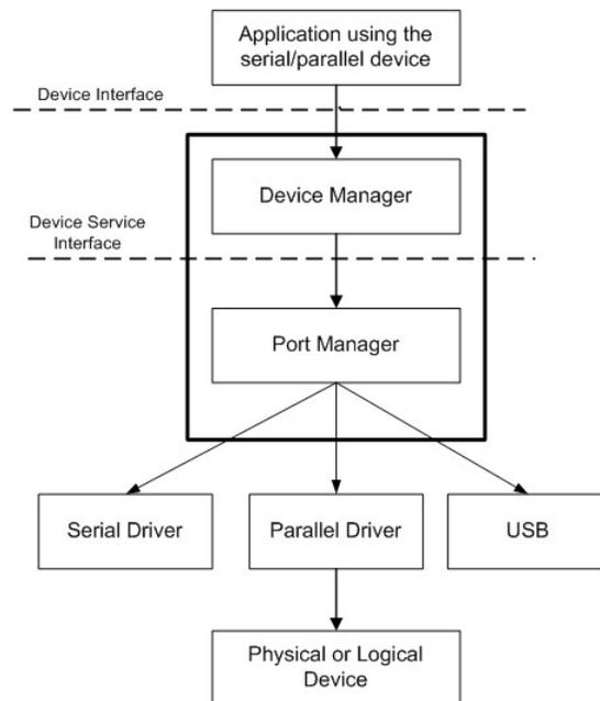
Figure 5.4: The structure of the Java Communication API [11]
