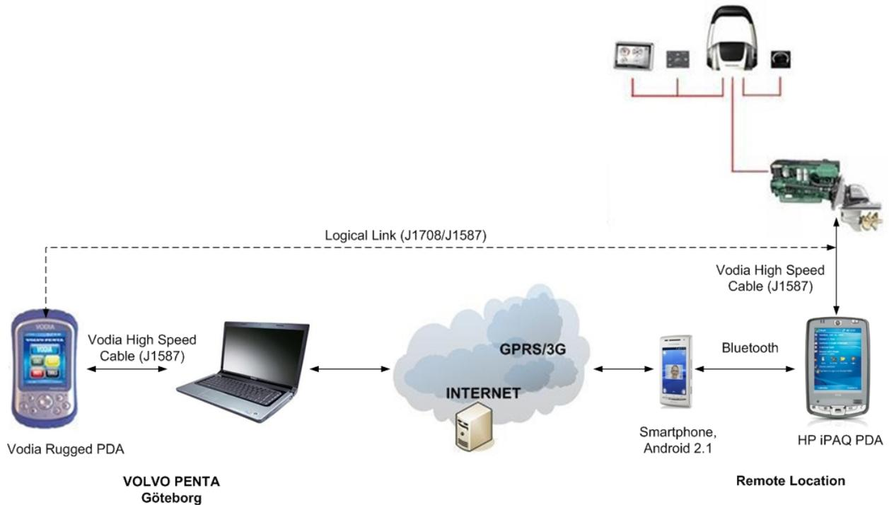
Figure 4.3: Possible architecture for the remote diagnostic system's prototype
