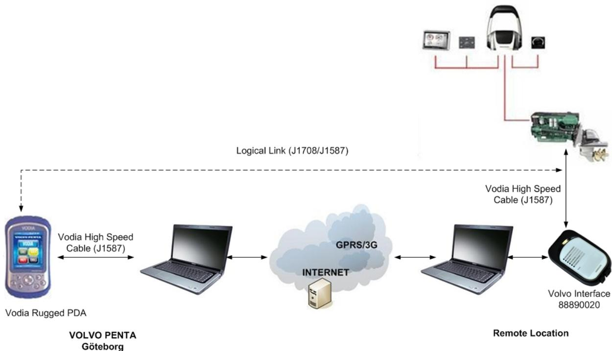
Figure 4.1: Possible architecture for the remote diagnostic system's prototype
