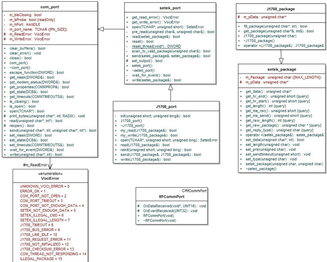
Figure 4.8: The class diagram for the PDA application
