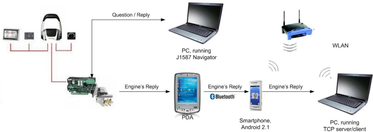
Figure 6.3: Hardware setup used for testing the PDA application
