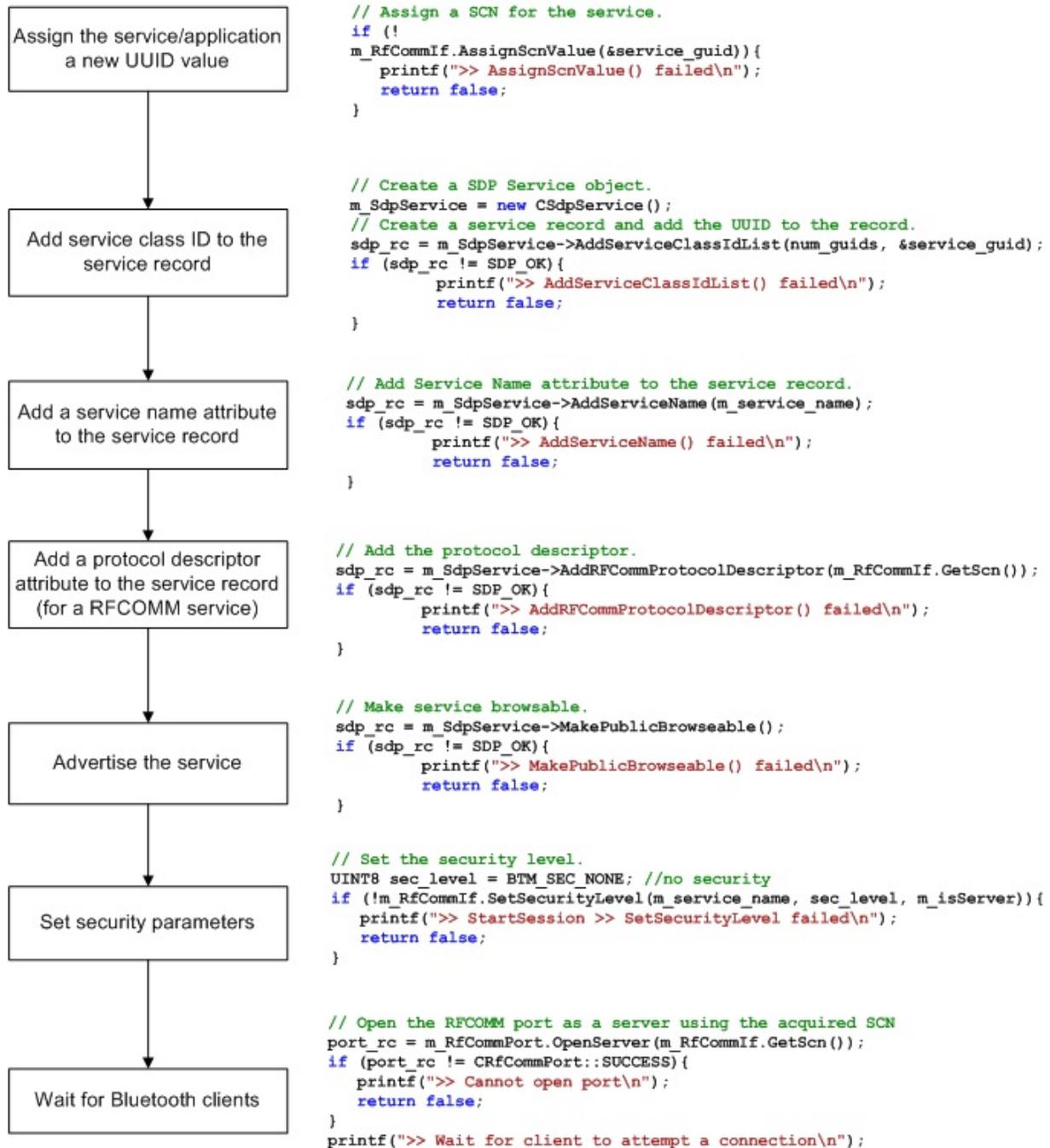
Figure 5.3: Steps for setting up a Bluetooth server application
