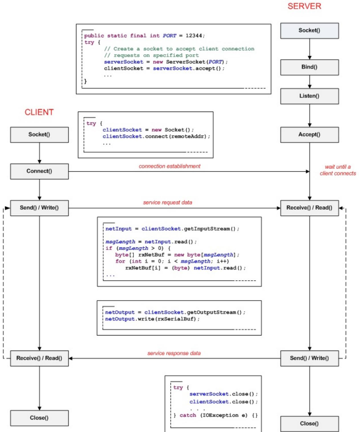
Figure 2.5: Client/Server applications scenario based on connection oriented protocols (Socket stream TCP)[5]
