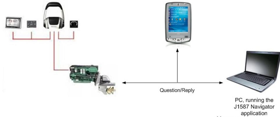
Figure 6.2: Hardware setup used for testing the PDA’s serial communication with the engine
