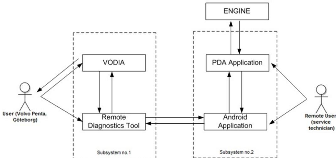
Figure 4.4: Prototype's conceptual architecture (Block diagram)
