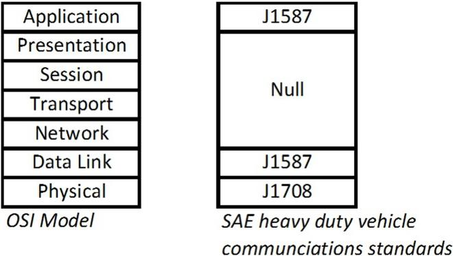
Figure 2.1: OSI reference model and the SAE standards
