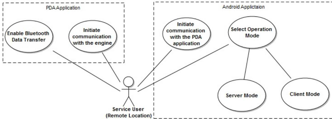
Figure 4.6: Use case diagram of the remote subsystem
