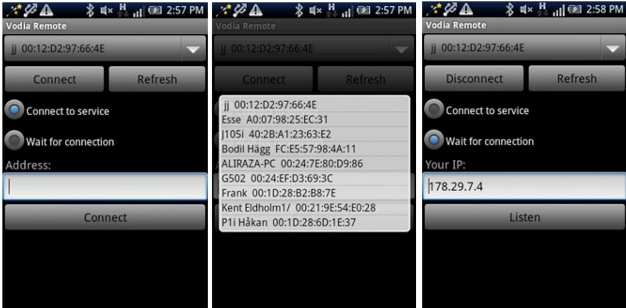
Figure 5.1: The user interface of the Android application at different connection phases. The first picture displays the general view, the second - the Bluetooth devices available in the local area and the third – the enabling of the server operation mode.
