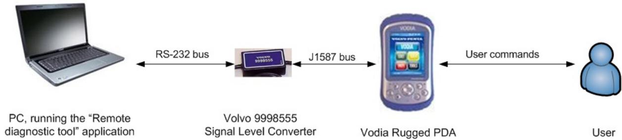
Figure 6.4: Hardware setup used for testing the "Remote diagnostic tool" – desktop application
