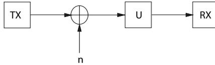
**Figure 3.2:** Simplified system model for  $k$  spans
