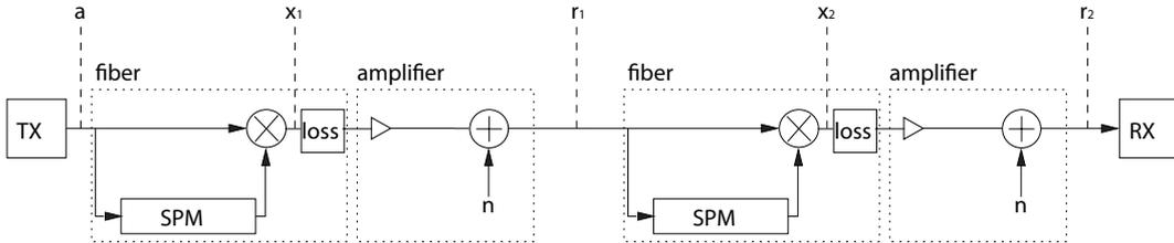
Figure 2.3: Transmission model for 2 spans.
