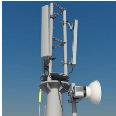
Figure 1.2: A typical base station having a set of transceiver antennas for communication between user terminal and network. Along with the transceiver is the microwave link, which carries the user data from the BS to BSC. Both the antennas are mounted either on a pole or tower at a specific height[2]
