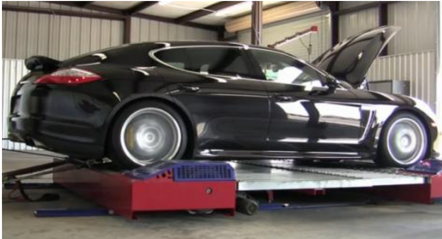
Figure 2.1 Dynamometer chassis testing
