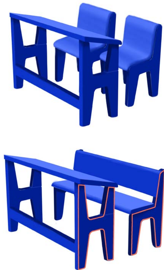
Figure 40. The same H-shaped side-module is used in both table and chair/bench.
