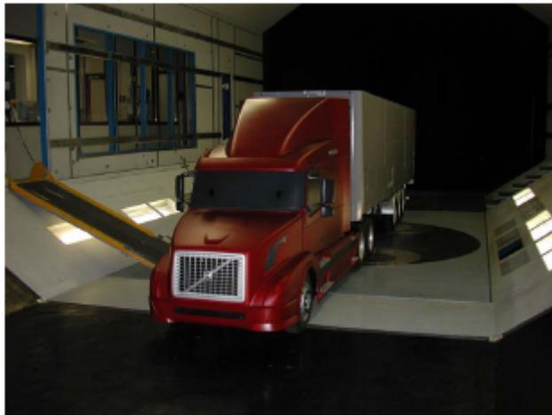
Figure 1.1.1: *An oscillating half-scaled Volvo truck in the RUAG wind tunnel.*
