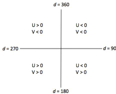
Fig 2.5 Quadrant where the wind direction belong is depending on value of  $U$  and  $V$  component [7].
