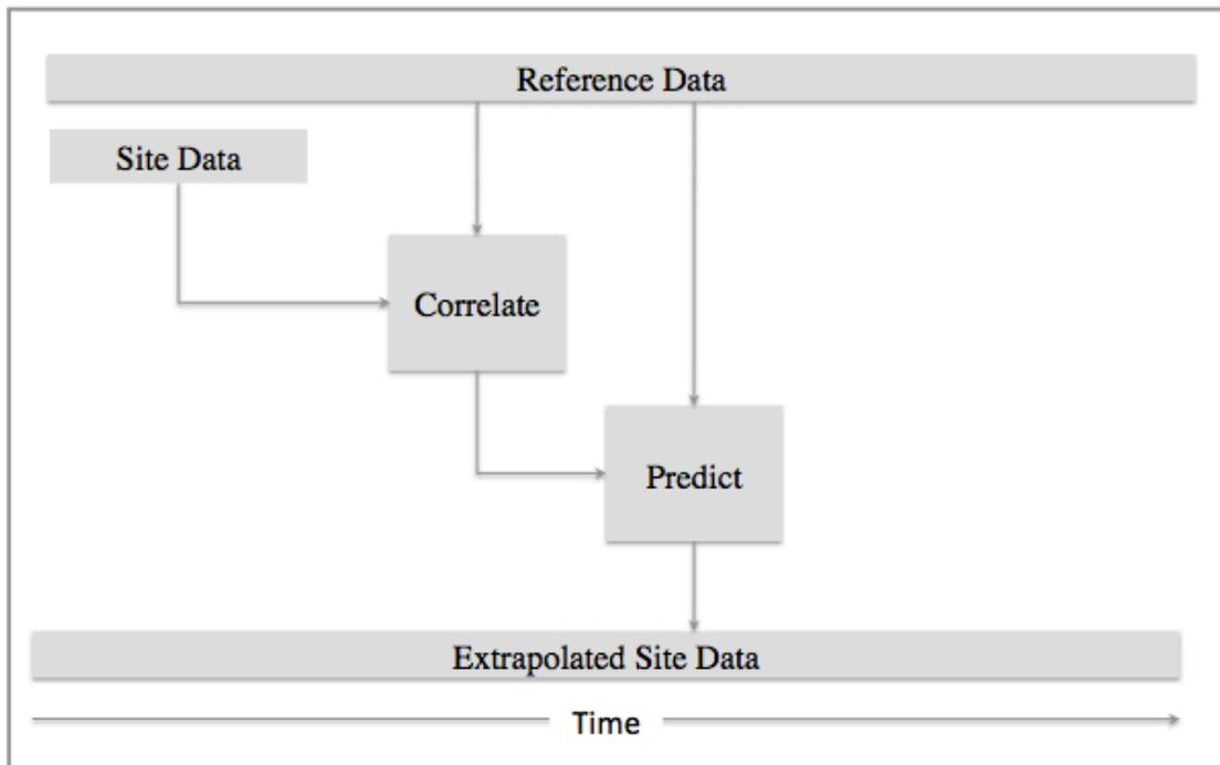
Fig 2.1 Scheme of the MCP procedure.
