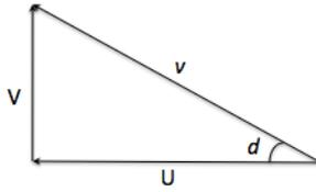
Fig 2.4  $U$  and  $V$  components of a wind vector.
