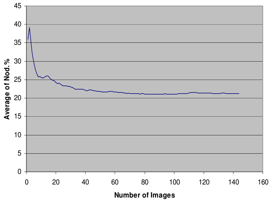
Figure 1. The average of nodularity versus the number of images for sample ATAS 5 based on the Volvo method.
