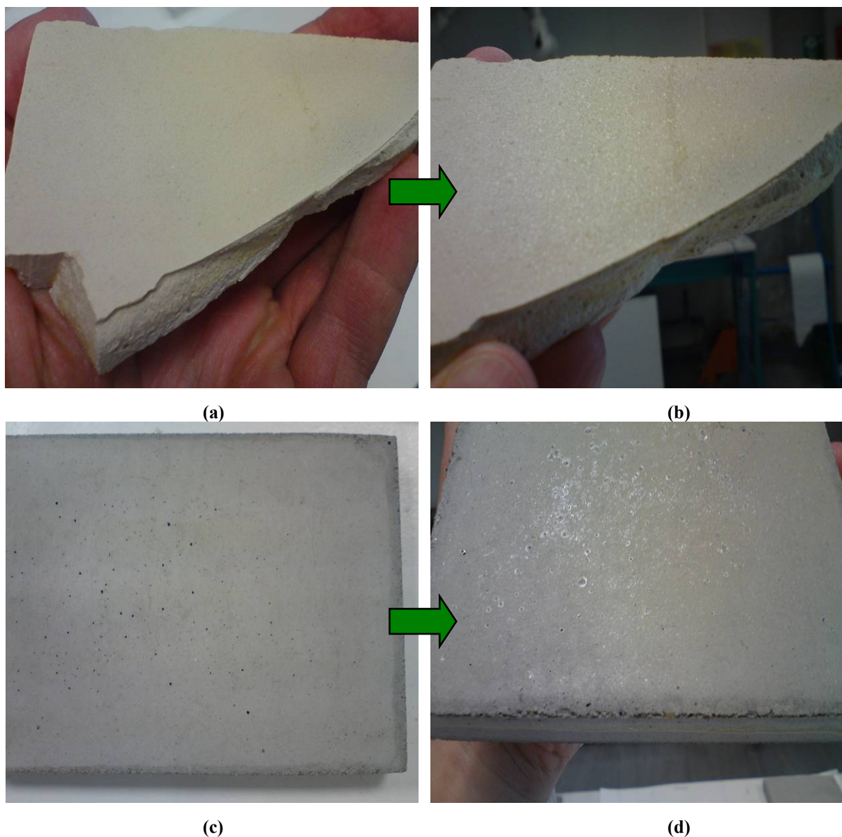
Figure 5.3.1 Dip-coating of chitosan 652 + 1% acetic acid on plaster and ordinary concrete in different chitosan 652 concentrations: (a) and (c) 1% chitosan while (b) and (d) 7% chitosan .
