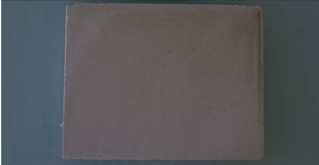
Figure 5.1.6 View of UHPC surface after deposition of coating
