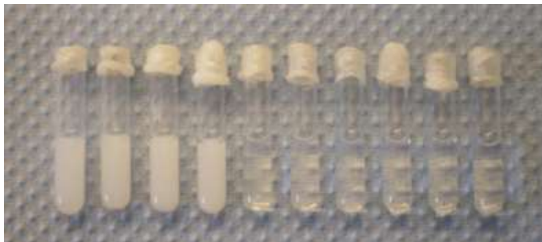
Figure 8 10 glass tubes witch containing constant silica with different salt content from 0.9 M in the left to 0.01 M in the right
