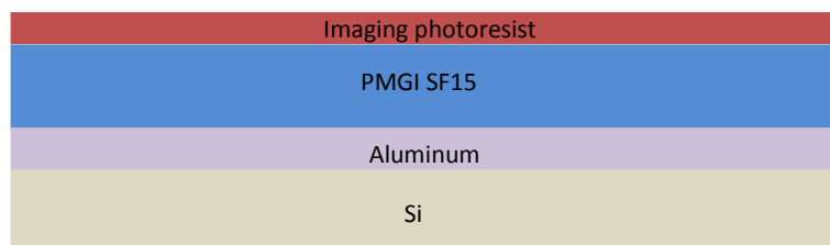
Fig.5.2 (b): Imaging photoresist S1813 coating on top of PMGI SF15.
