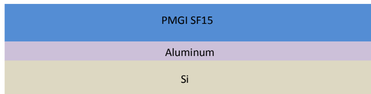
Fig.5.2 (a): PMGI SF15 coating on top of aluminum.
