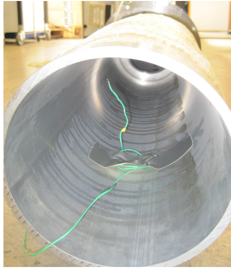
Figure 6.5: The green cable is the thermo couple placed inside the tube with the orifice in the background
