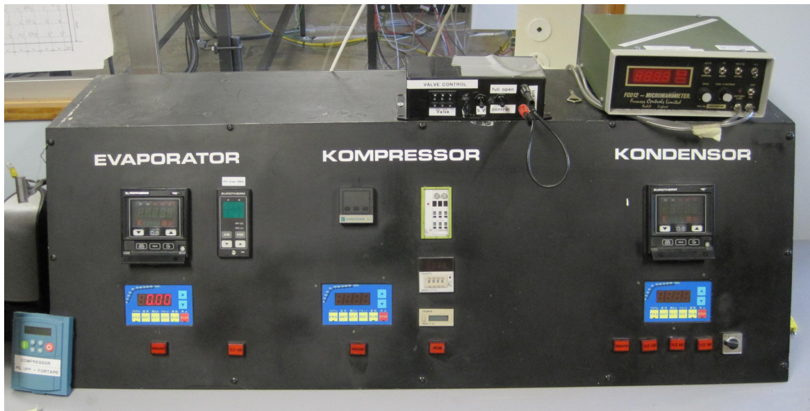
Figure 4.2: The old control panel of the HVAC test rig
