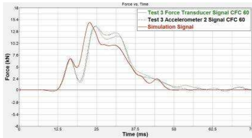
Figure 5.8 Force Vs Time phase 2 Test 03
