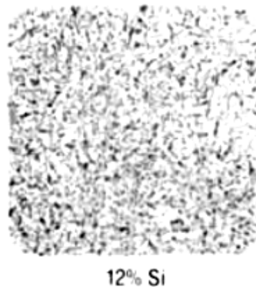
Figure 2.3 Microstructure of cast AlSi12 alloy
